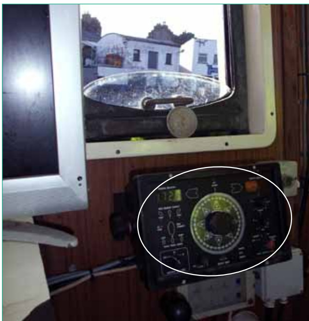
Position of autopilot in relation to the wheelhouse starboard window
