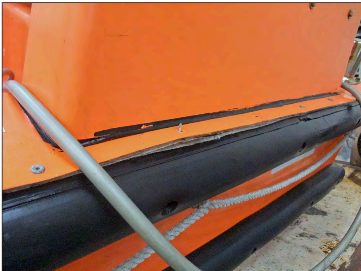
Figure 3: Failure of rivets on port gunwale
