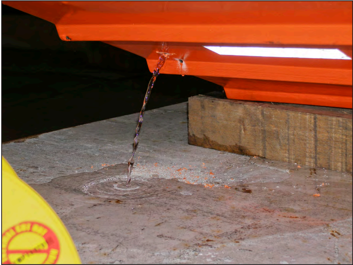
Figure 12: Water draining from drilled hole
