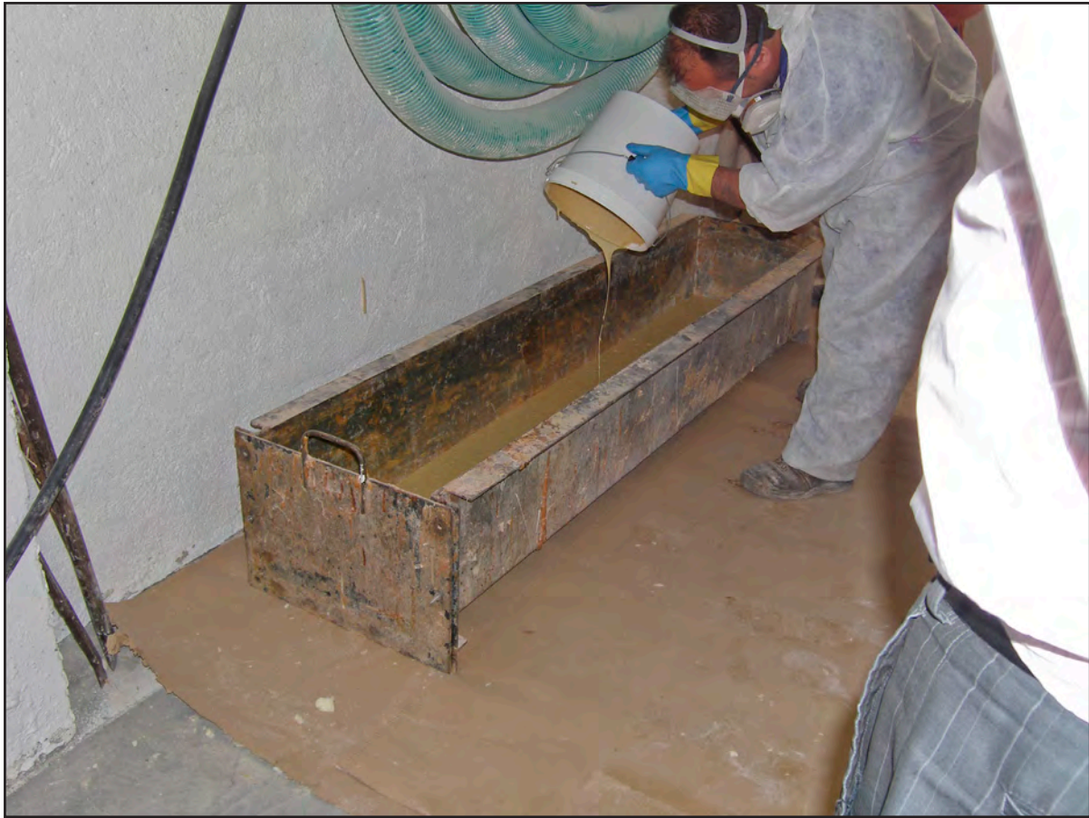
Figure 23: Pouring foam mix into mould
