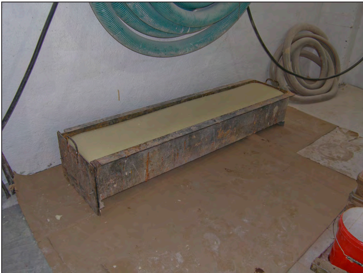
Figure 24: Foam expanding in mould
