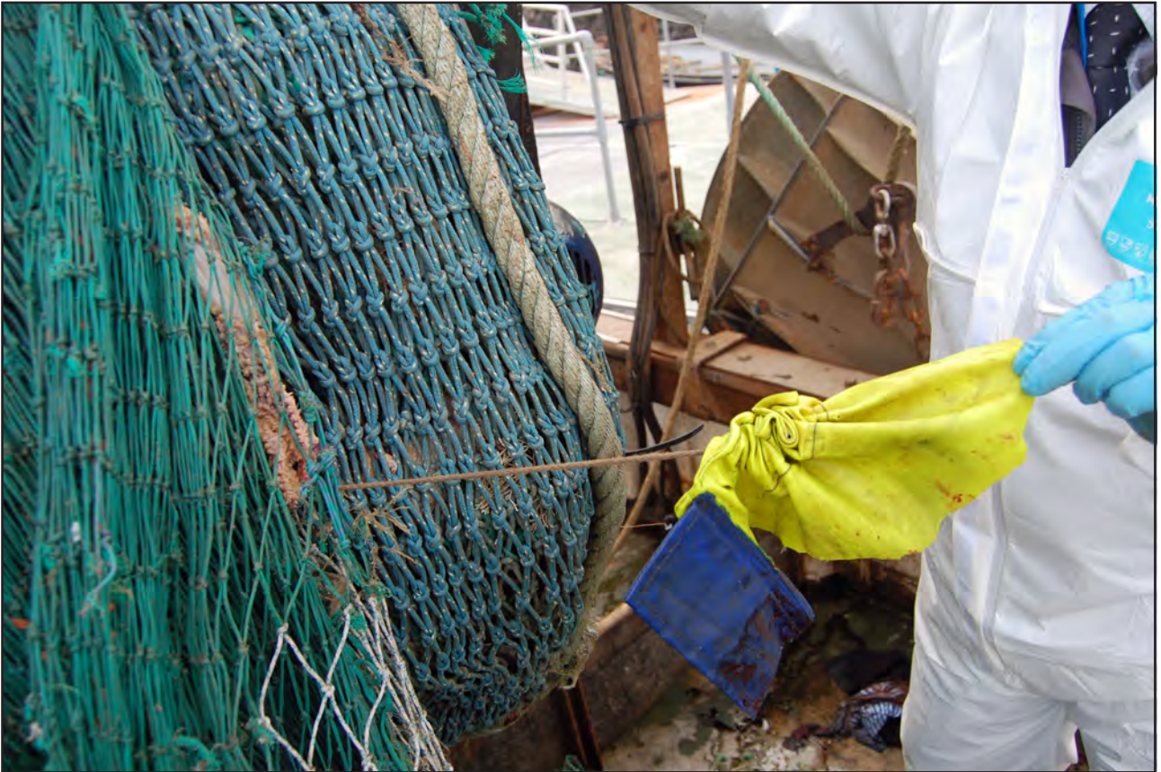
Partial storm hood and drawstring leading across to port drum
