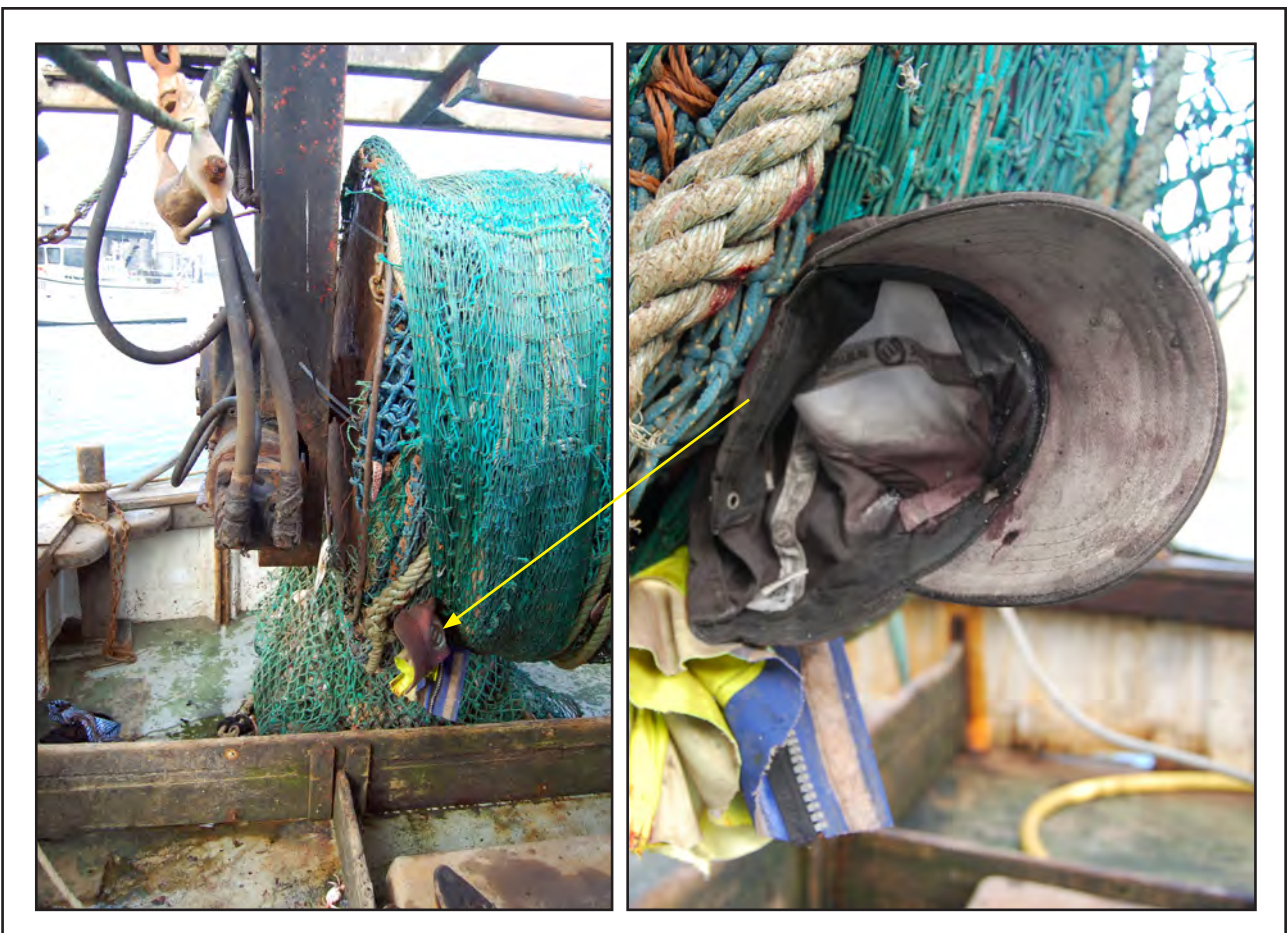
Net drum showing location of trapped cap and partial jacket
