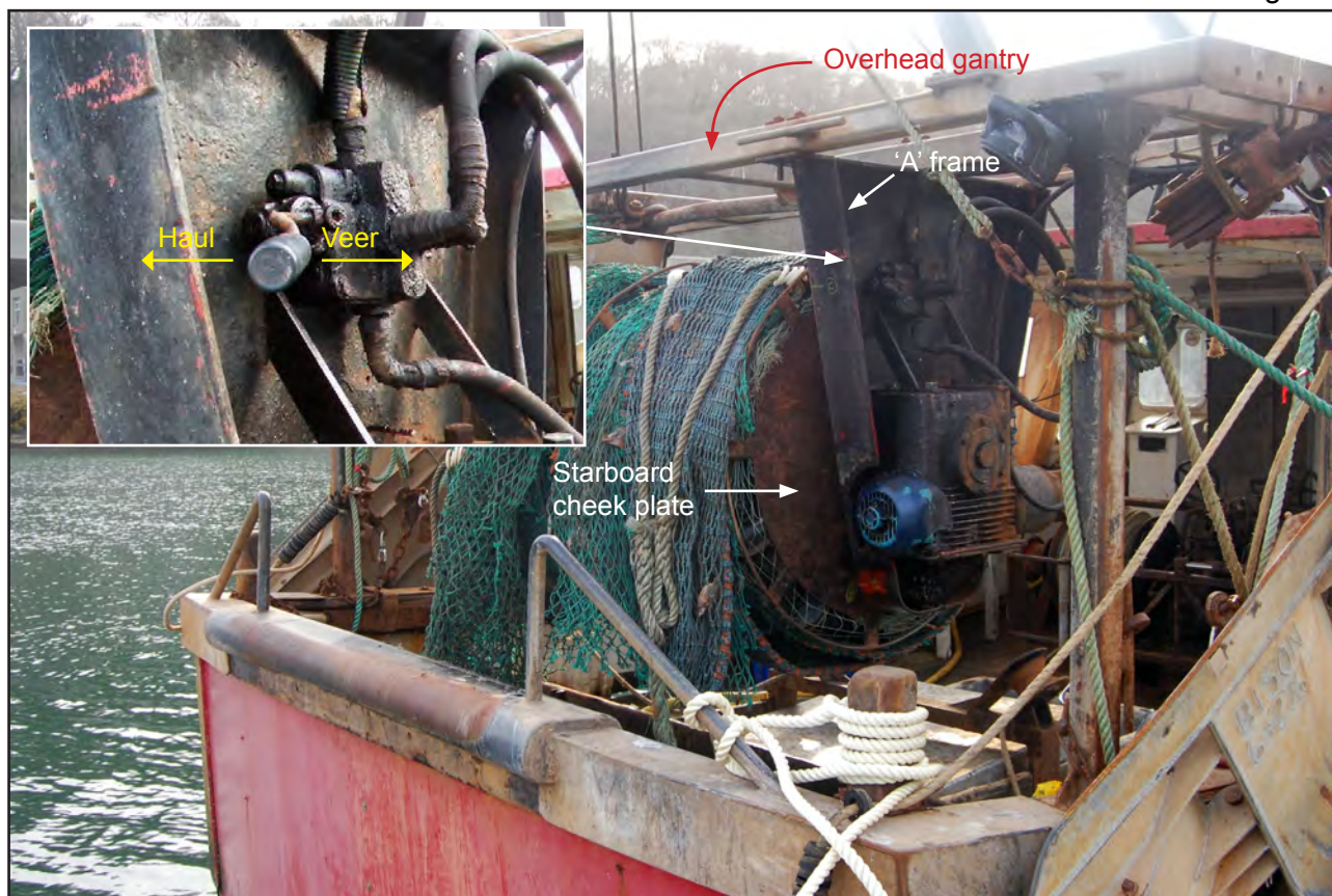
Net drum - showing location of control lever
