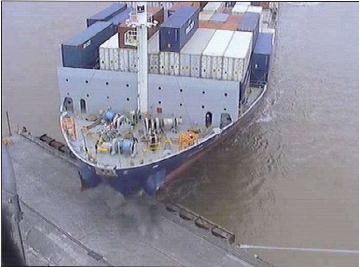
CCTV image showing contact with quay
