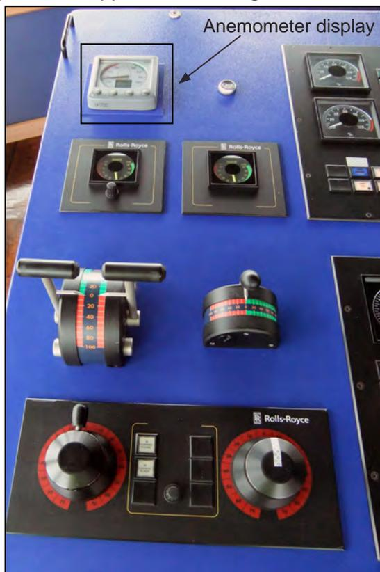
**Figure 13:** Bridge wing wind indicator
