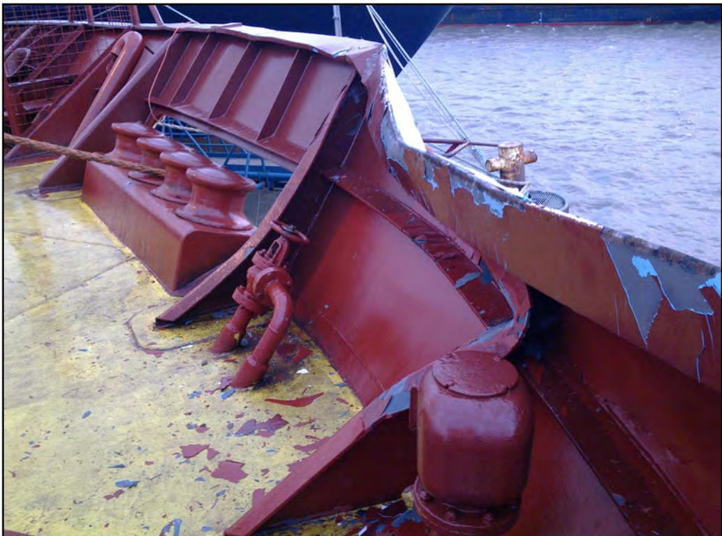
**Figure 10: Damage to Scotia Seaways**
