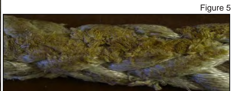
Section of the failure zone showing extreme abrasion damage
