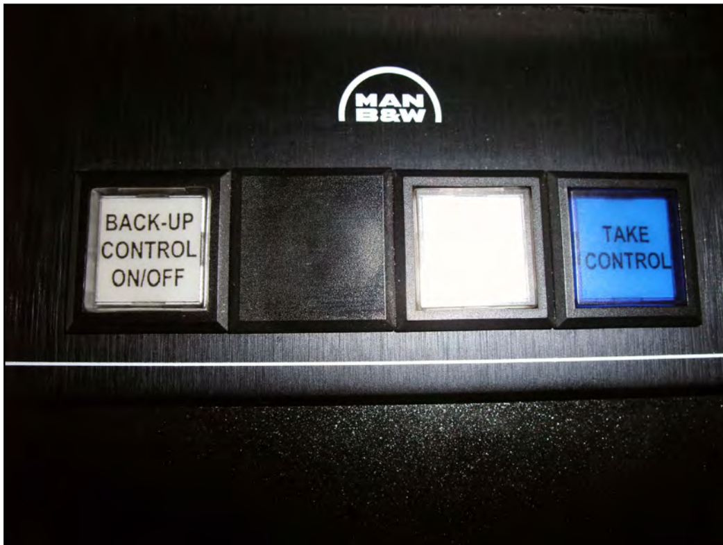
Figure 7: Backup control to bypass the AT2000 PCS
