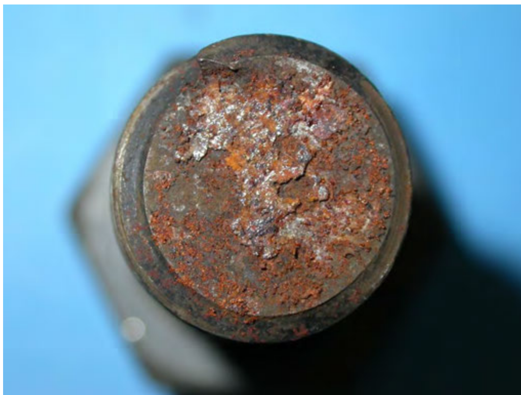
Figure 15: Threaded bolt half exhibiting fatigue like fracture and showing heavy rusting of the fracture surface.
