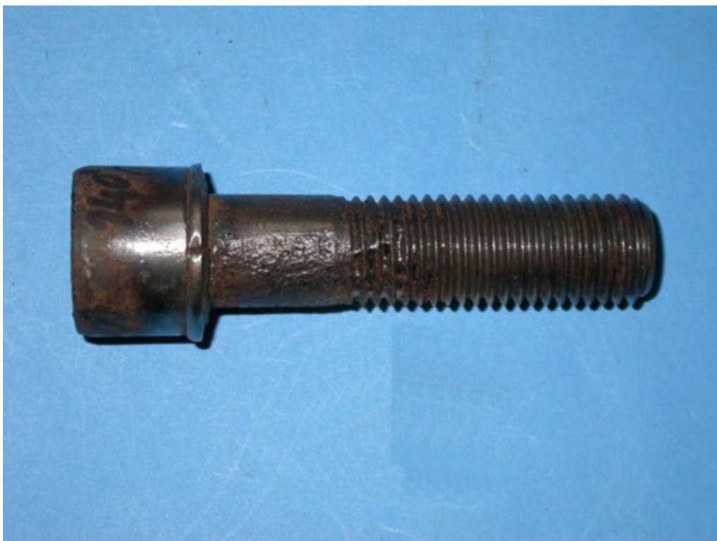
Figure 12: Un-fractured bolt, shown after cleaning and exhibiting evidence of local pitting corrosion.
