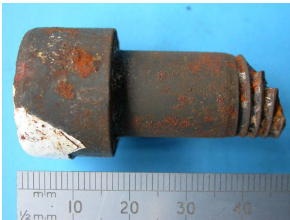
Figure 2: Detail of figure 1, showing bolt half exhibiting 45° degree shear like fracture.
