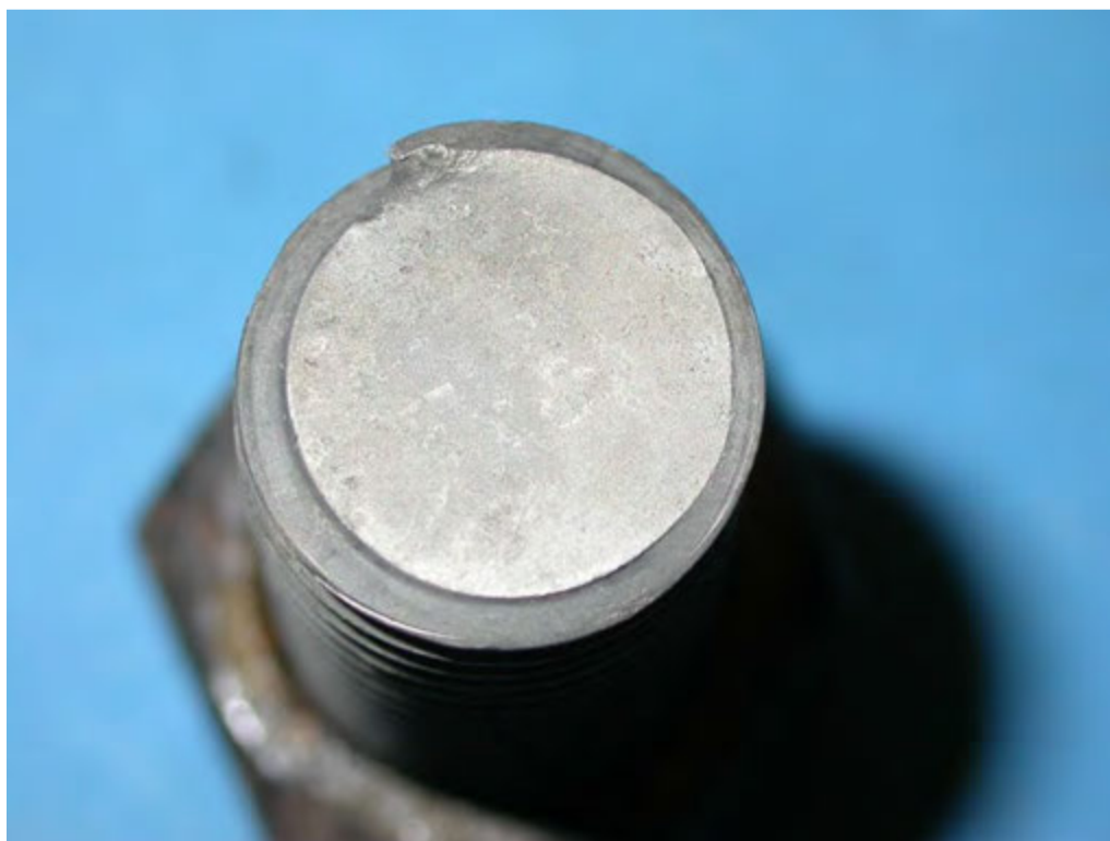
Figure 17: Second threaded bolt half exhibiting fatigue like fracture, shown after cleaning in Clarke solution.
