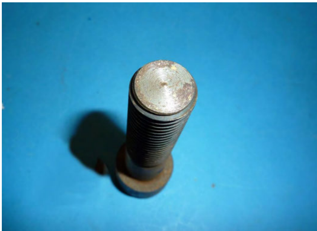
Figure 10: Second un-fractured bolt, showing evidence of prior plating at its threaded end.
