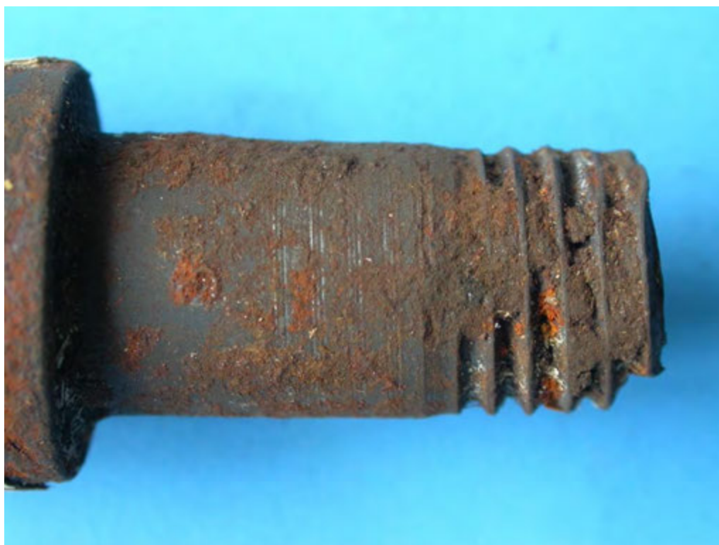
Figure 4: Detail of figure 1, showing a bolt half exhibiting fatigue like fracture at 90° to the fasteners principal axis.
