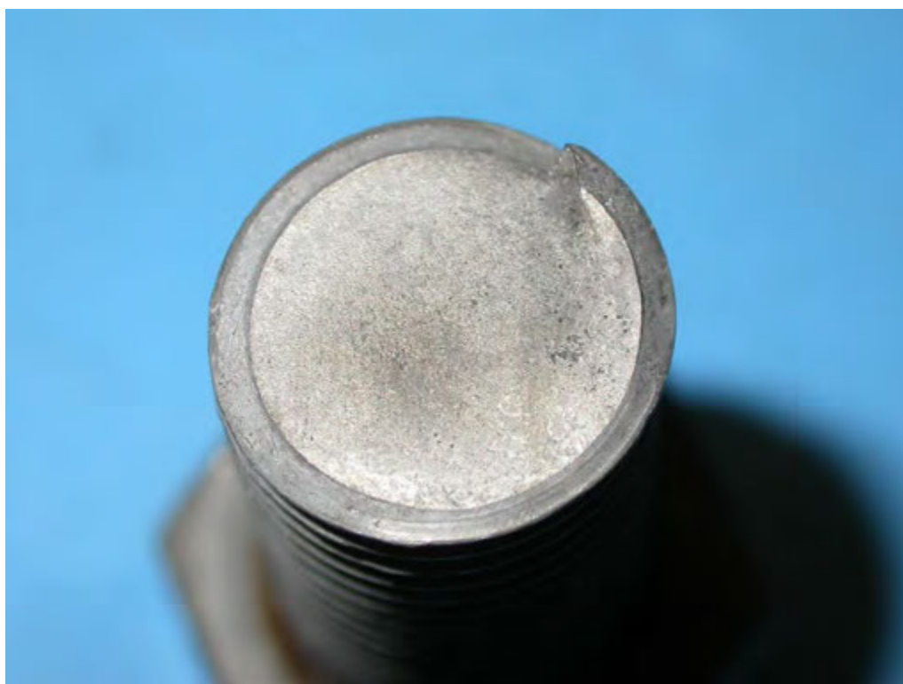
Figure 16: Threaded bolt half exhibiting fatigue like fracture, shown after cleaning in Clarke solution.
