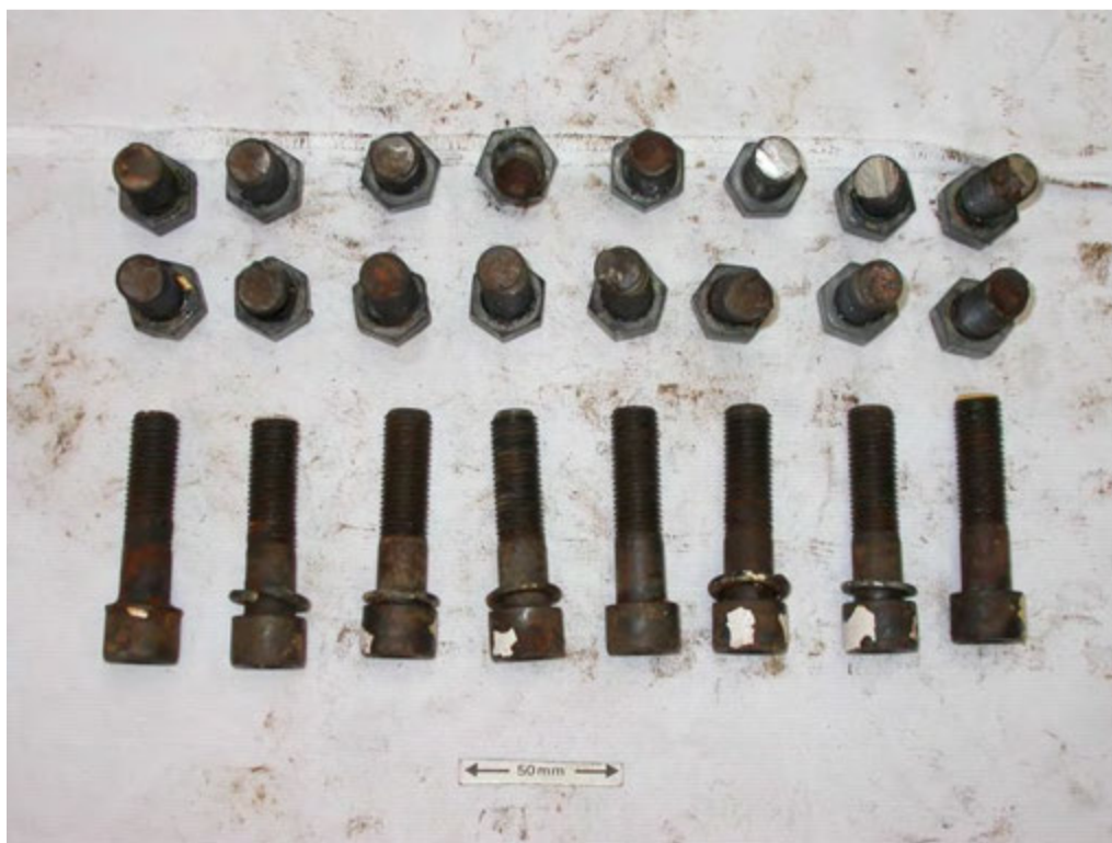
Figure 7: Bolt samples received 8 th August, showing 8 un-fractured, 4 exhibiting 45° shear like fractures, 10 exhibiting fatigue like fractures and 2 with sawn faces.
