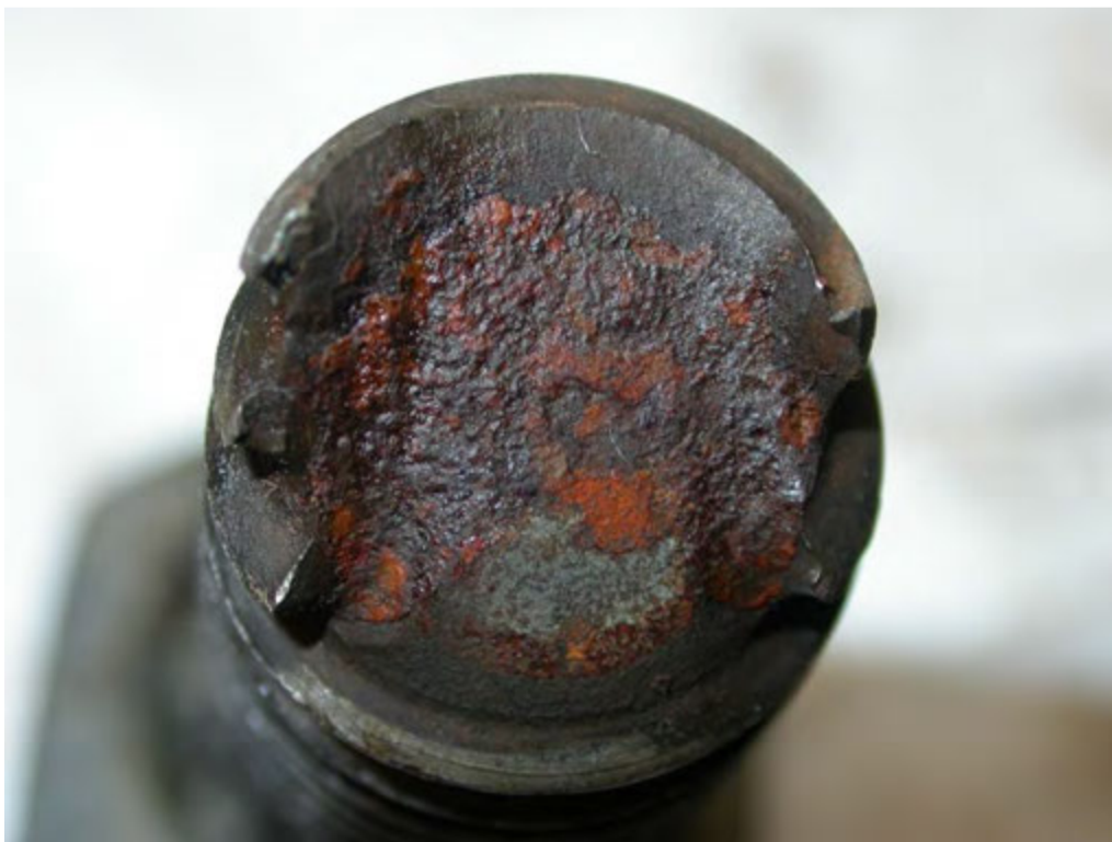
Figure 19: Second threaded bolt half exhibiting 45° shear like fracture and showing moderate rusting.
