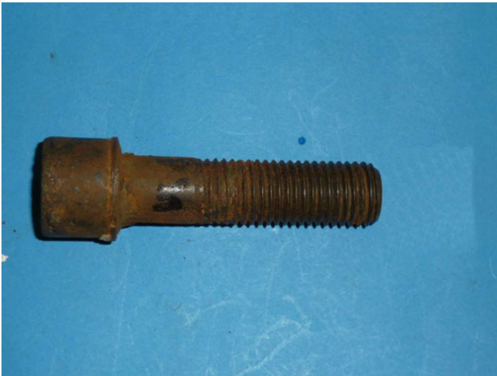
Figure 11: Un-fractured bolt showing external corrosion.
