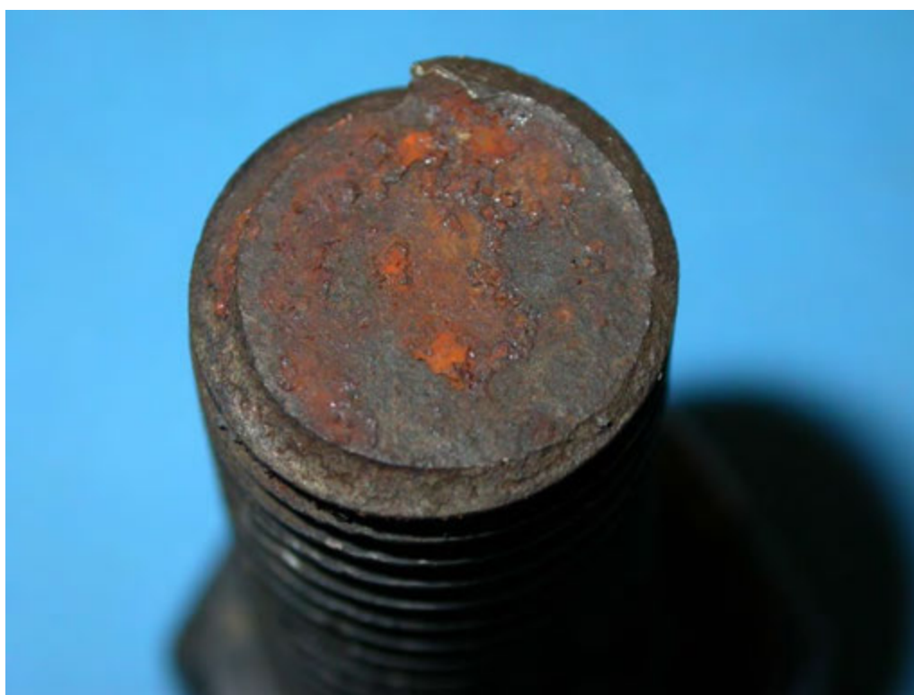
Figure 14: Threaded bolt half exhibiting fatigue like fracture and showing moderate rusting of the fracture surface.
