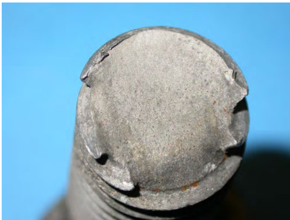
Figure 21: Second threaded bolt half exhibiting 45° shear like fracture, shown after cleaning in Clarke solution.
