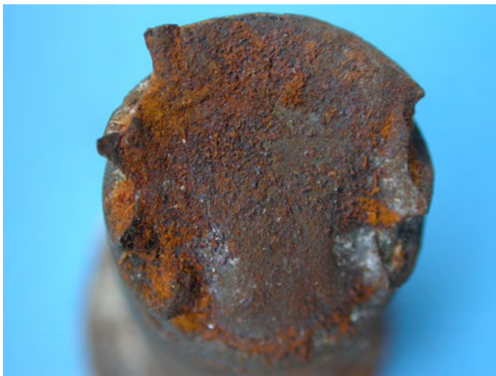
Figure 3: Detail of figure 1, showing rusted fracture surface of the bolt half exhibiting a shear like fracture.
