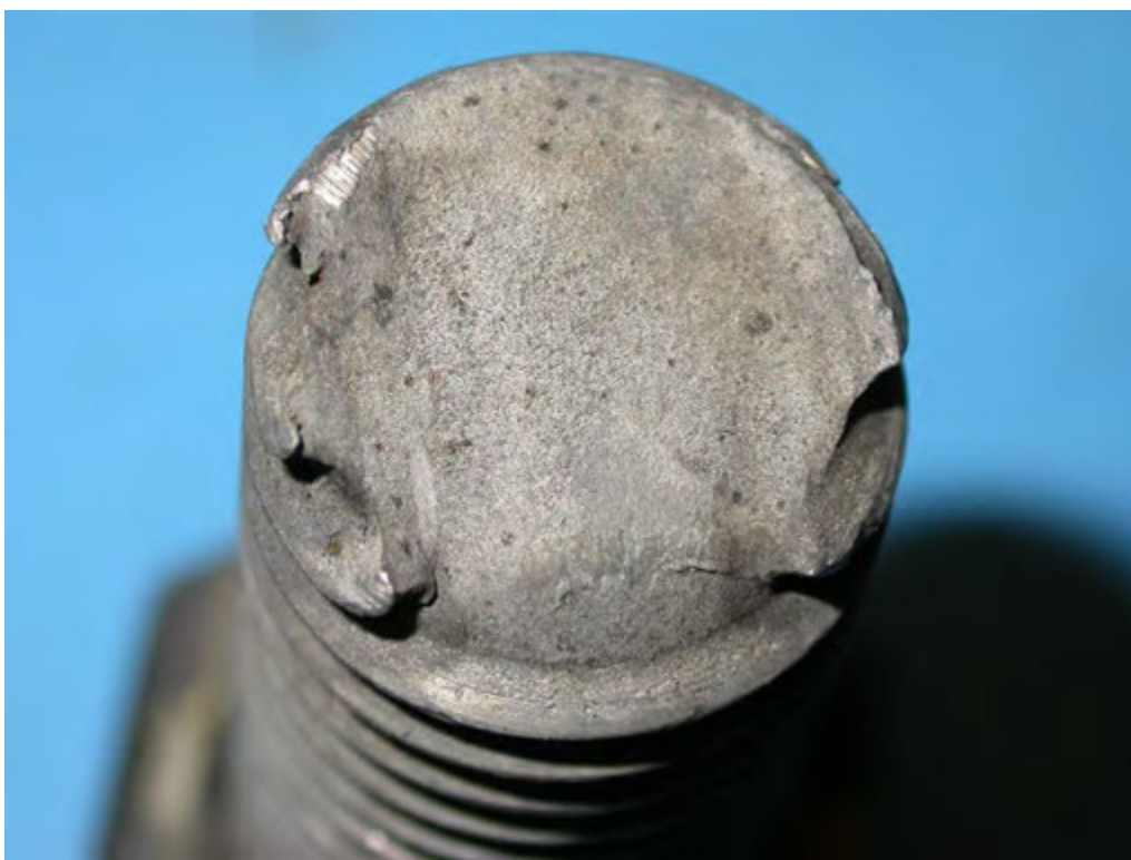
Figure 20: Threaded bolt half exhibiting 45° shear like fracture, shown after cleaning in Clarke solution.
