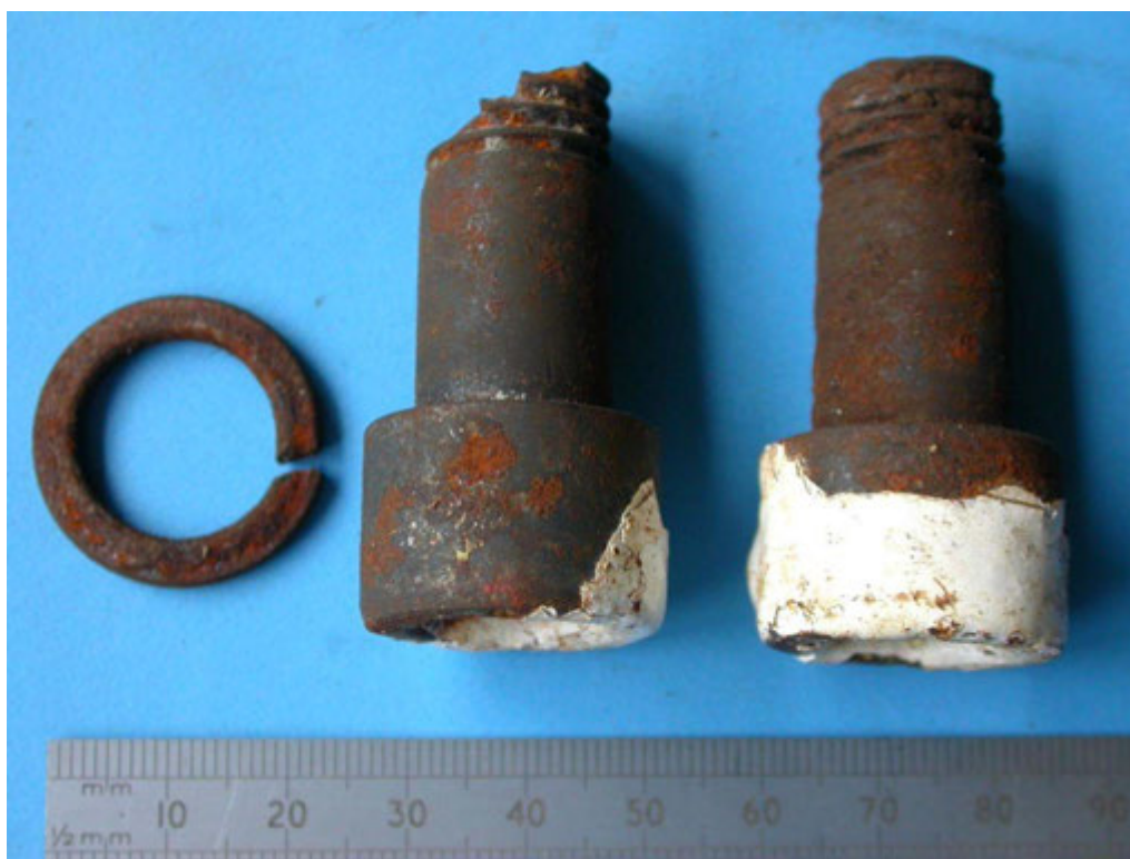
Figure 1: Fractured cap head bolt sample halves, received 3 rd August 2011.
