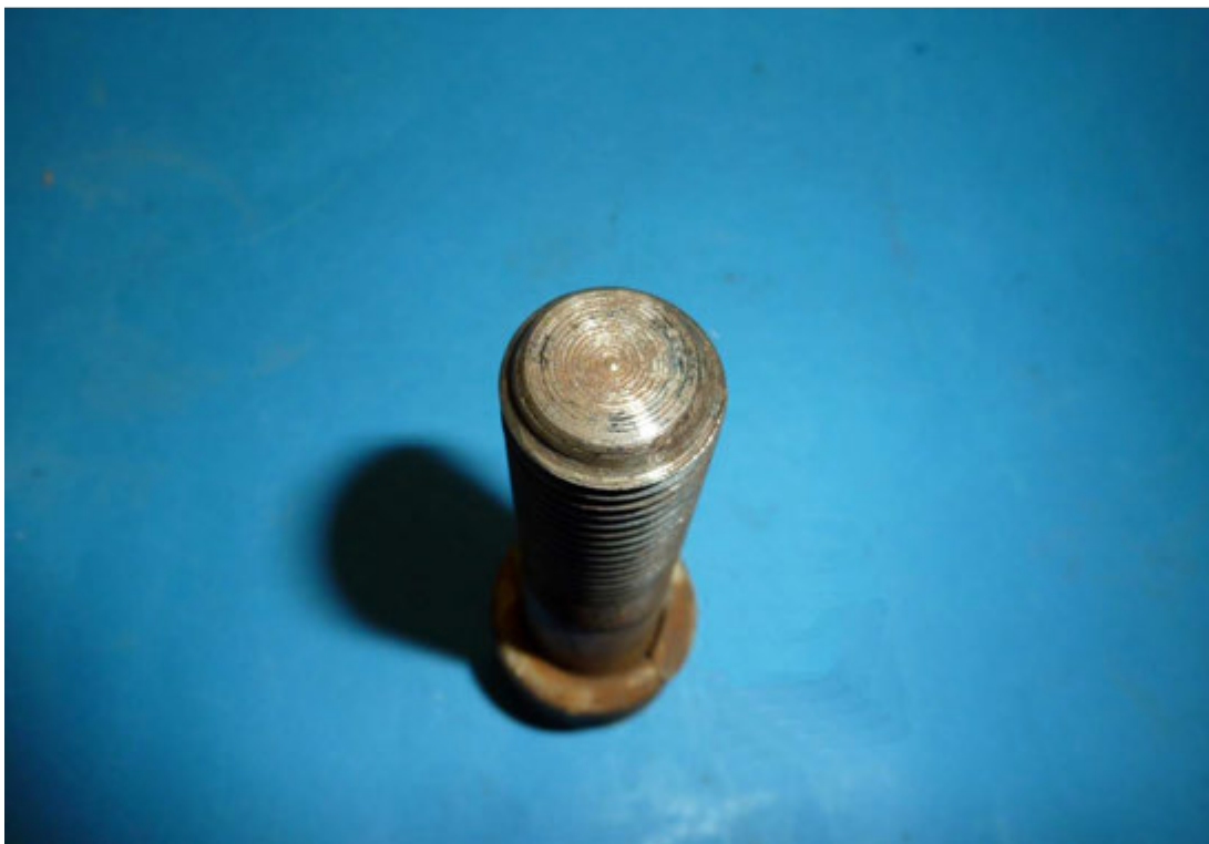
Figure 9: Un-fractured bolt, showing evidence of prior plating at its threaded end.
