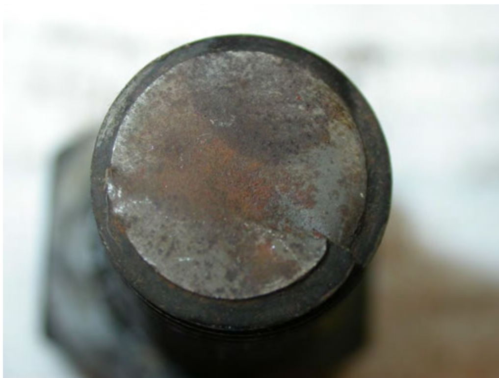
Figure 13: Threaded bolt half exhibiting fatigue like fracture and showing light rusting of the fracture surface.
