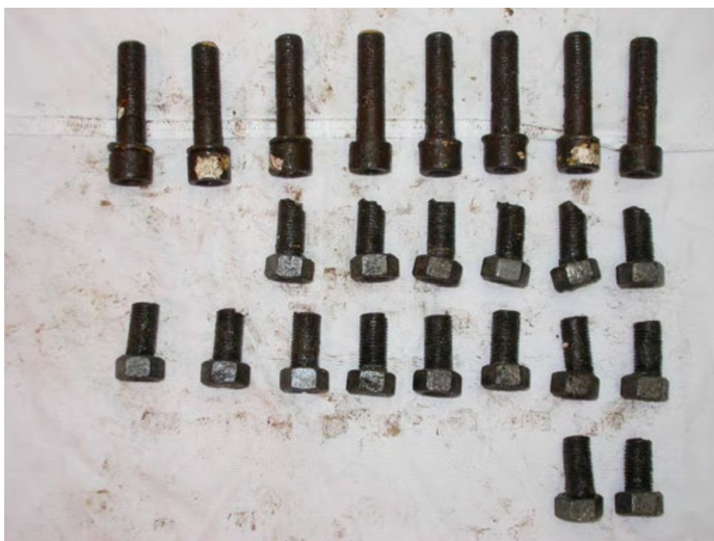
Figure 6: Un-fractured cap head and threaded end bolt fracture halves received 8 th August 2011.
