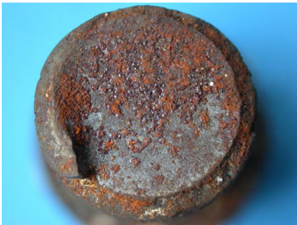
Figure 5: Detail of figure 1, showing rusted fracture surface of the bolt half exhibiting a fatigue like fracture.
