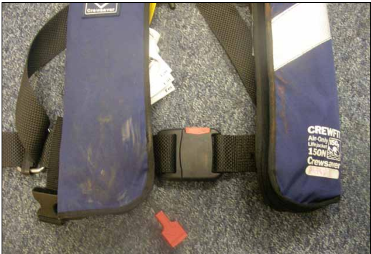
Figure 12: Bulwark rail paint residue on lifejacket
