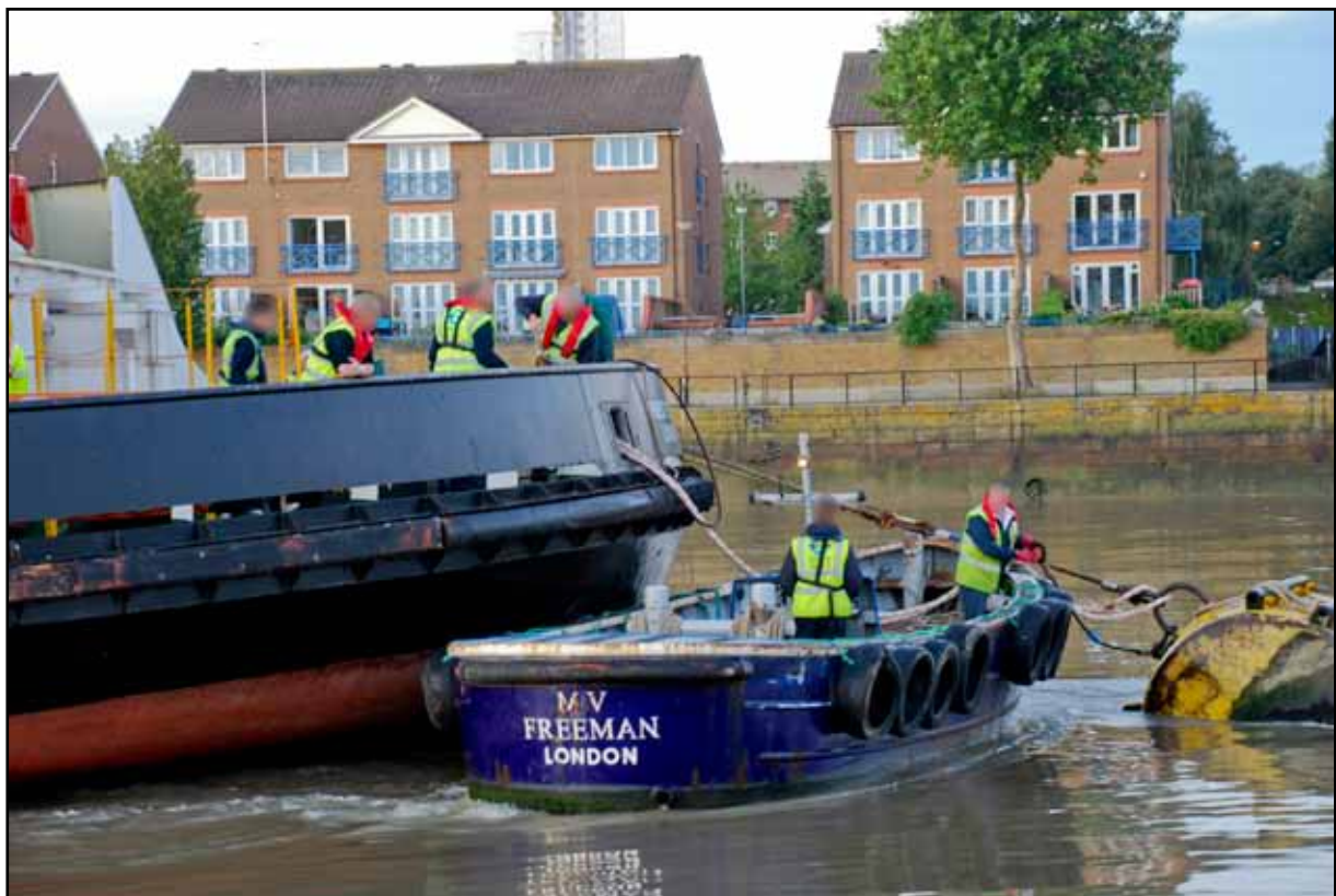
Figure 2: Mooring ropes and insurance wire being released by workboat
