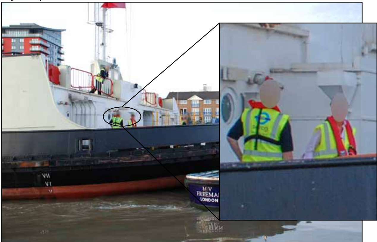
Figure 16: Serco staff member wearing lifejacket without crotch strap fitted
