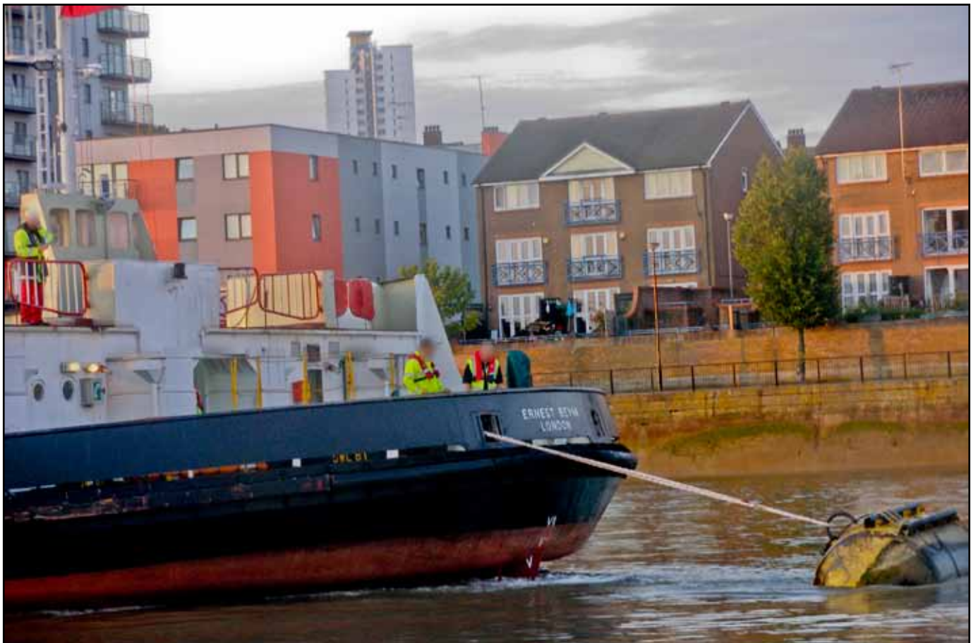
Figure 4: Ernest Bevin tethered by up-tide slip rope only
