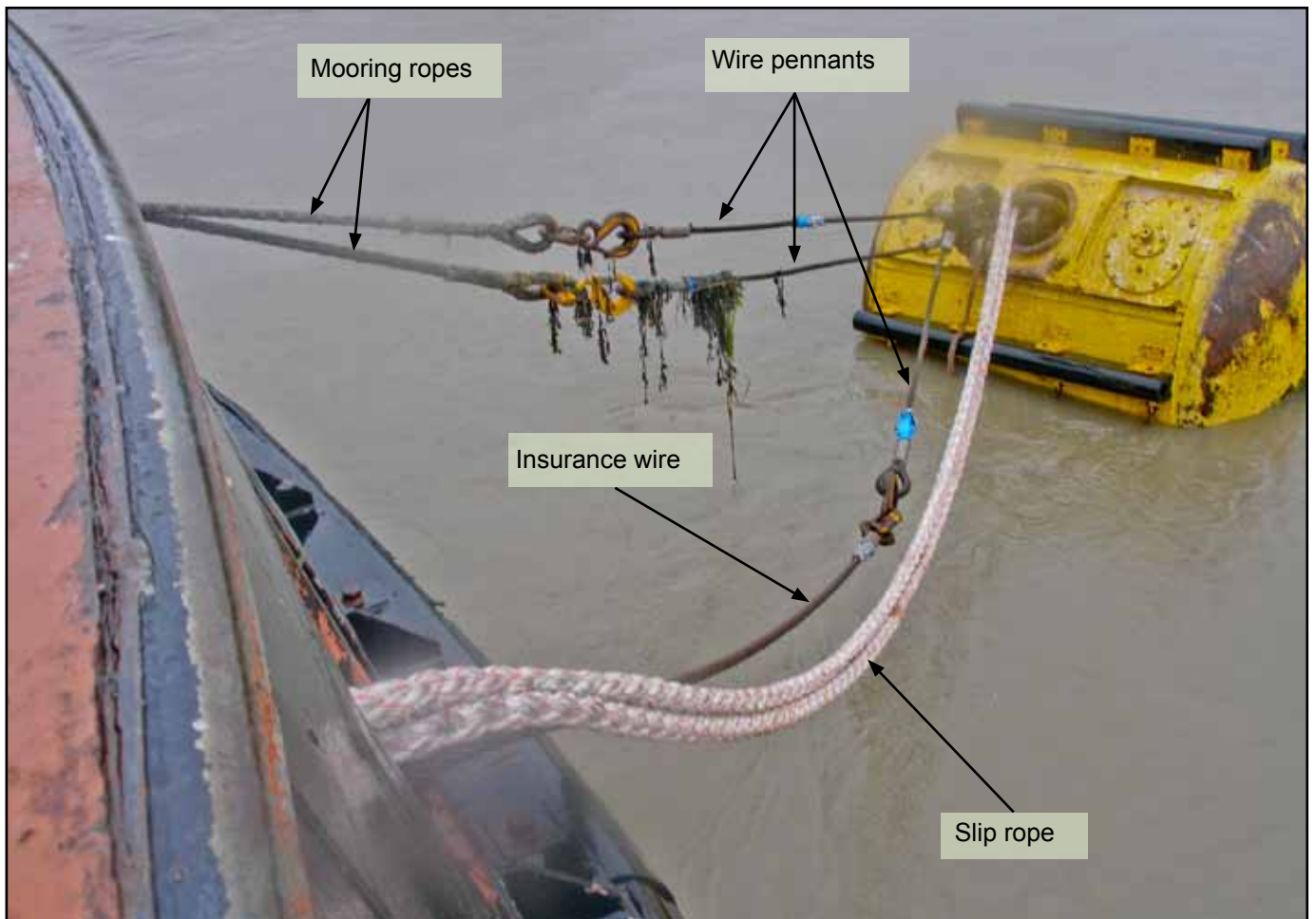
Figure 3: Various securing devices between Ernest Bevin and mooring buoy
