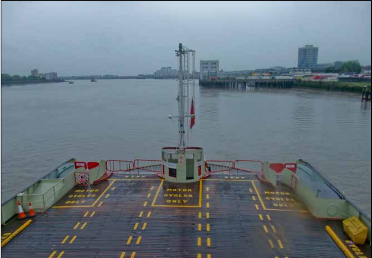
Figure 9: Master's view from control platform towards the mooring deck while moored to buoys (Note: The obstruction posed by the traffic control hut and the lack of visibility of the mooring buoy)
