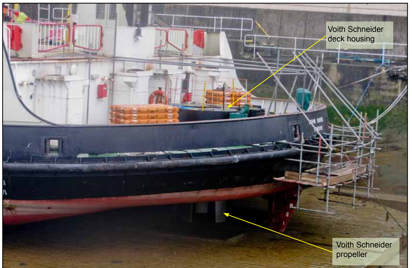
Figure 8: Sister ship John Burns showing Voith Schneider propeller below the counter
