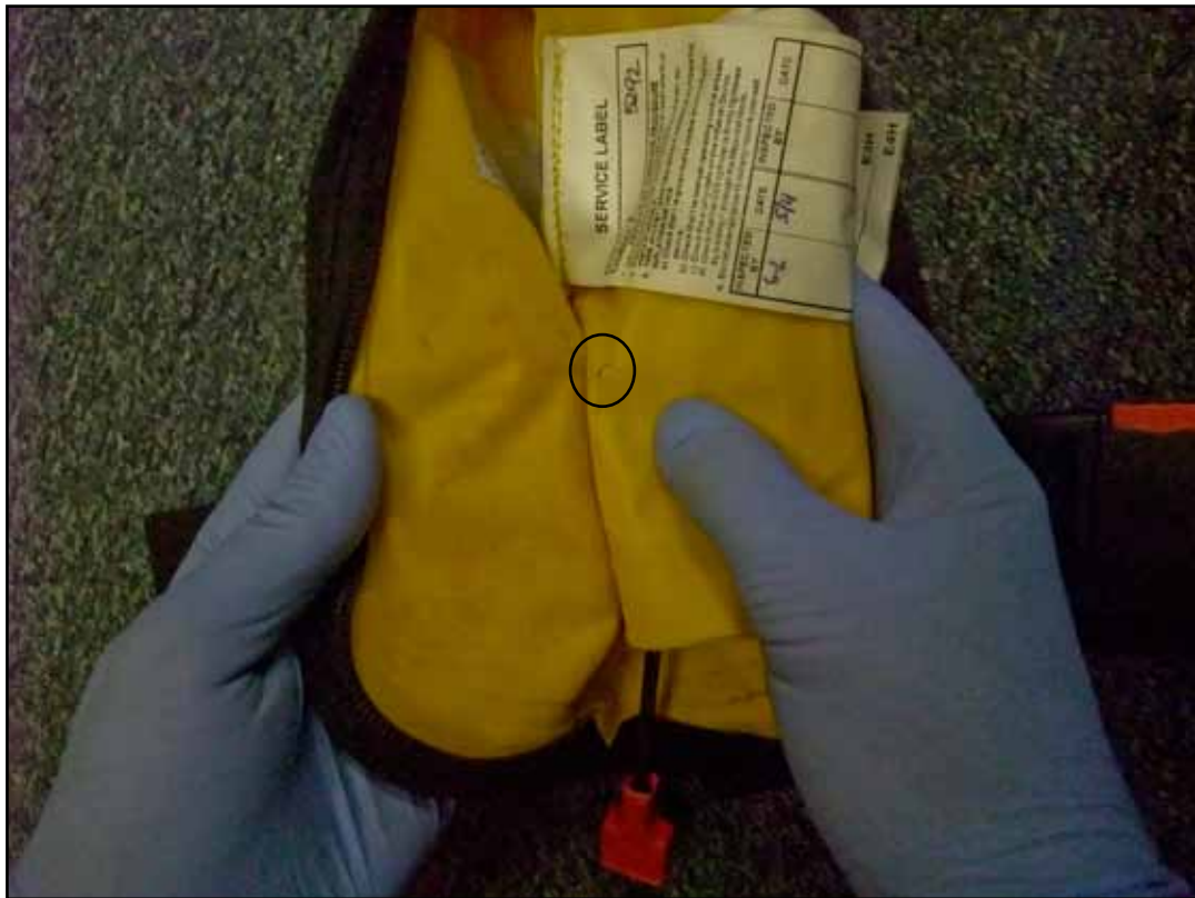
Figure 11b: Lifejacket puncture
