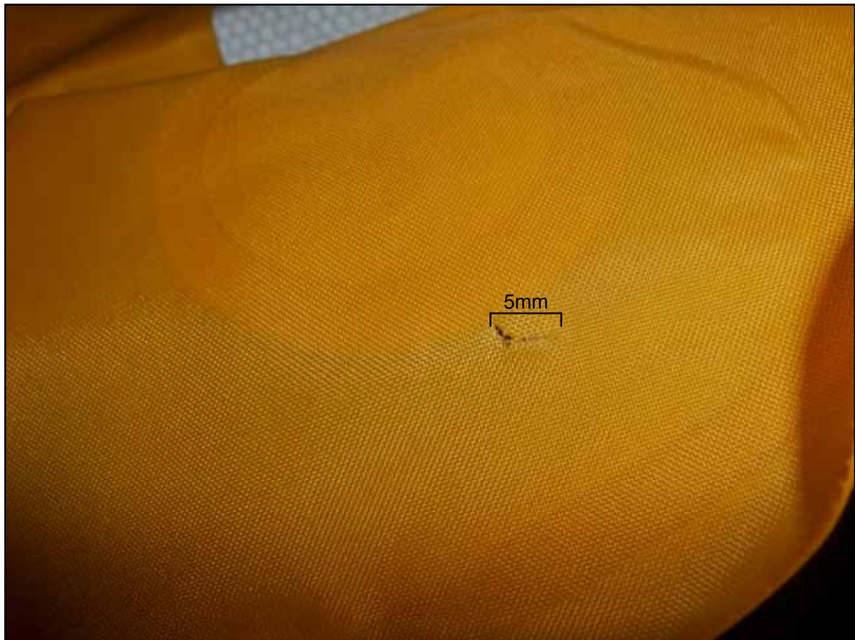
Figure 11a: Lifejacket puncture
