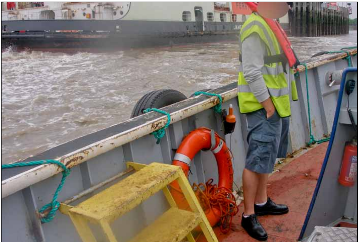
Figure 6b: Workboat deck and relative height of bulwark for manoverboard recovery
