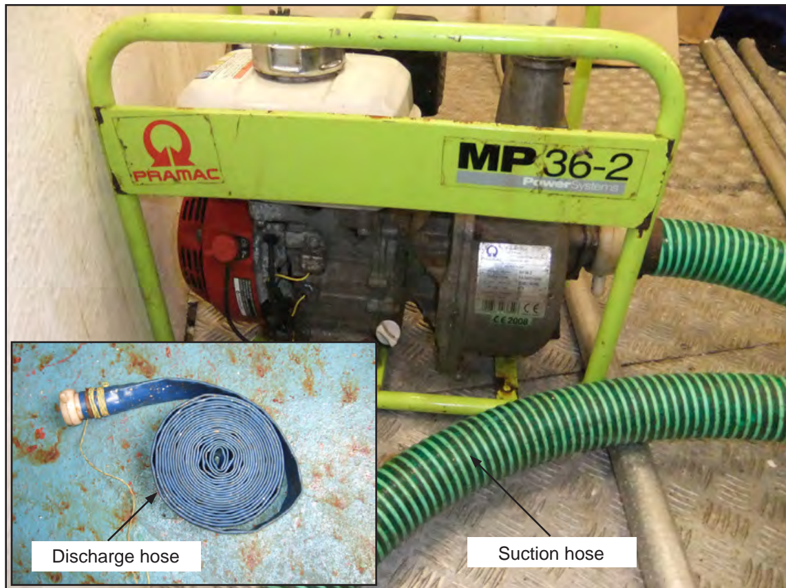
Figure 1: Starlight Rays' petrol engine-driven pump and hoses
