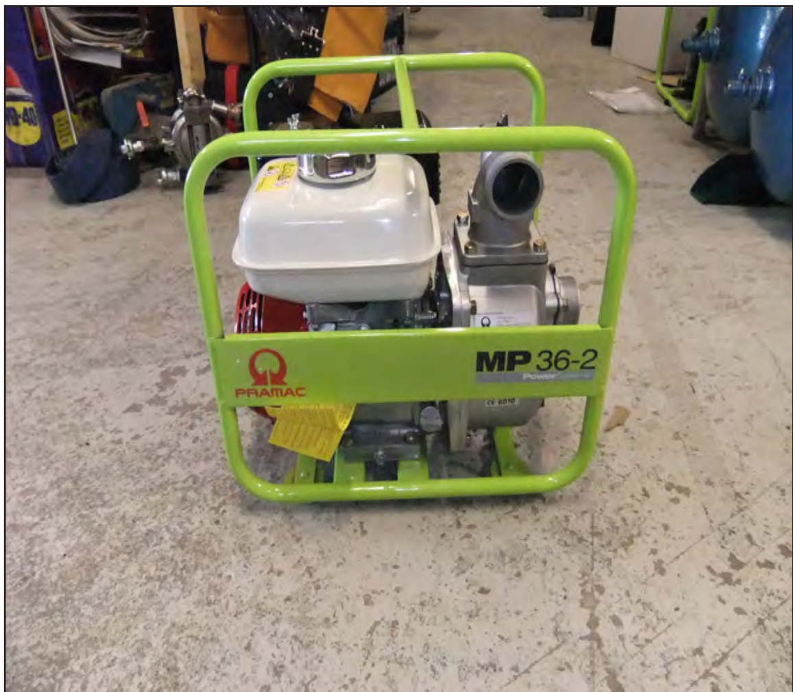
Figure 13a: Pramac MP 36-2 petrol engine-powered pump
