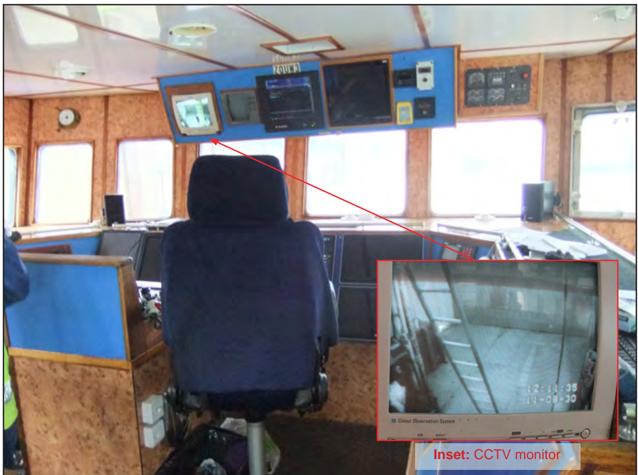
Figure 10: Wheelhouse watchkeeping chair, radar and inset, CCTV monitor display
