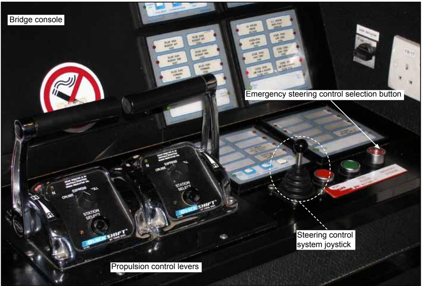
**Figure 2:** Steering control system joystick
