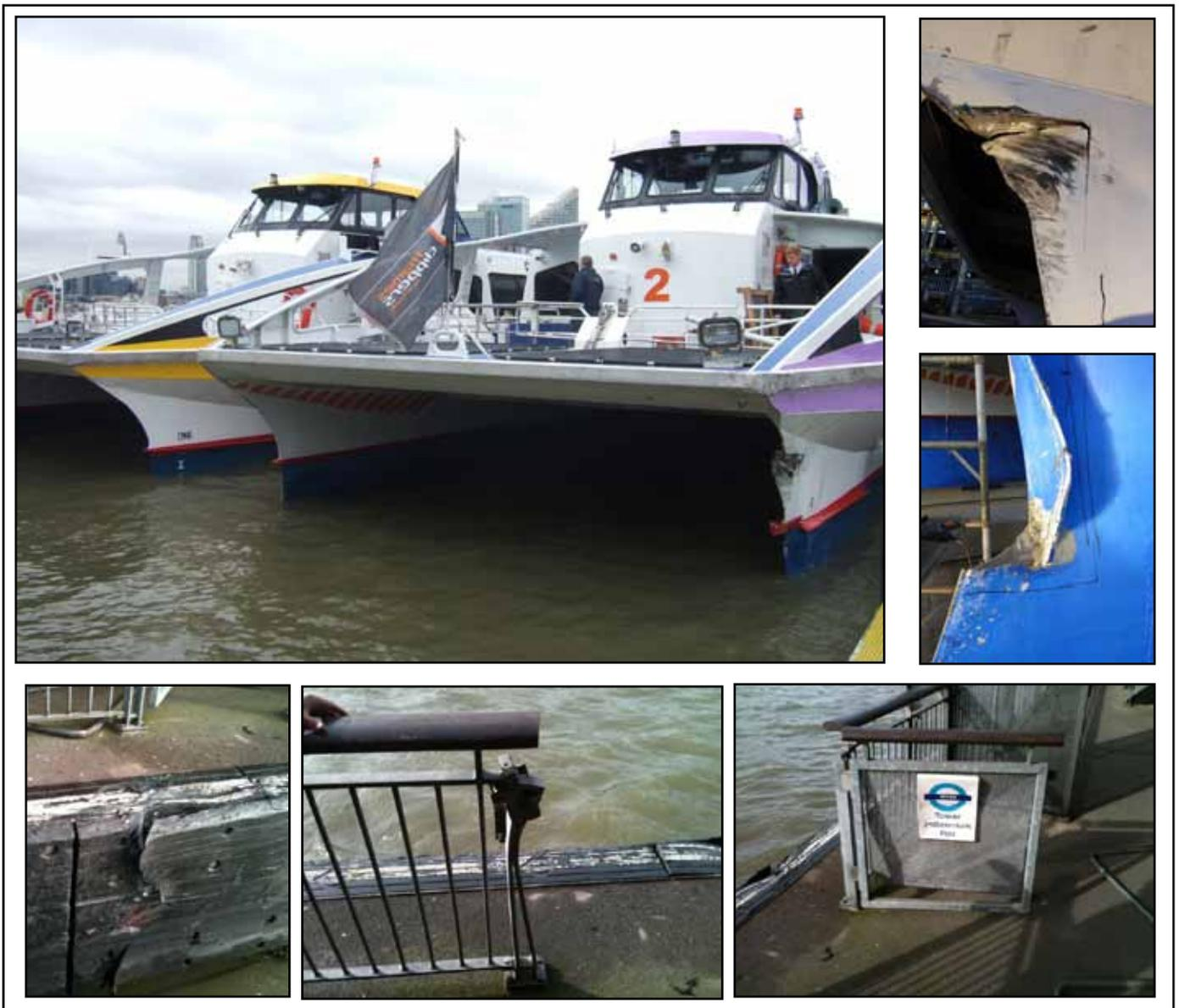
**Figure 12:** Damage caused by the contact
