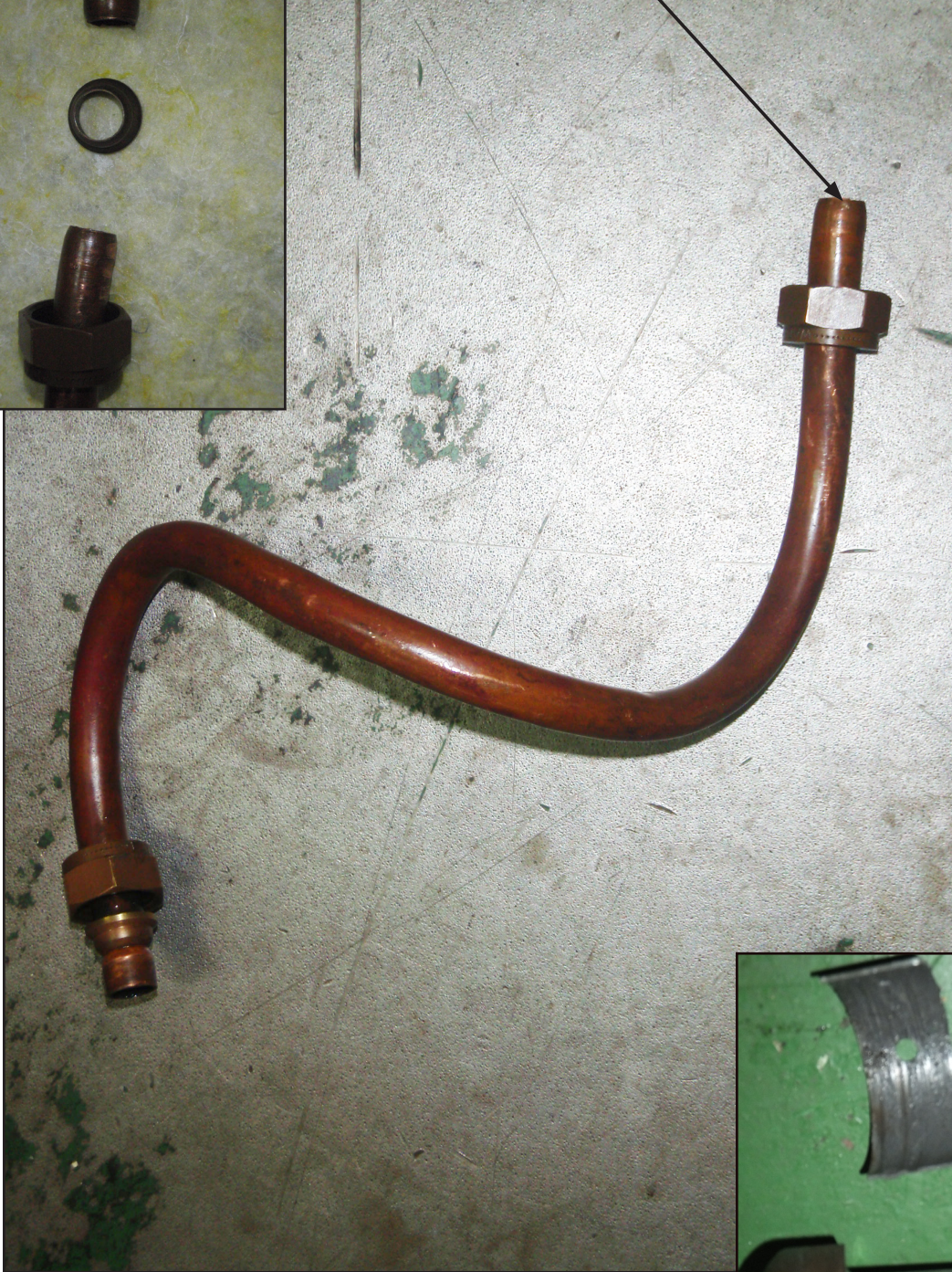
Failed lubricant oil pipe end fitting
