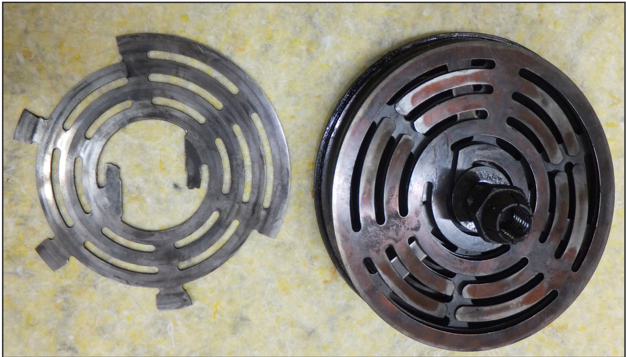
Figure 5: Damage to No 1 compressor, low pressure discharge valve
