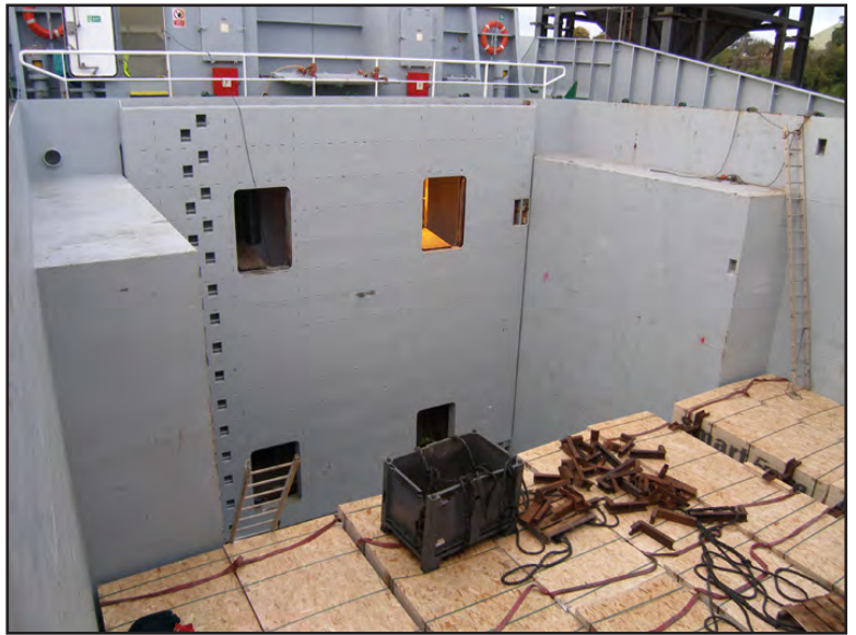
Figure 1: Forward portable bulkhead
