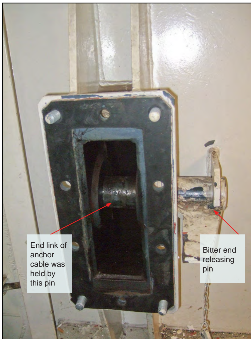
Figure 5: Releasing pin for bitter end of port anchor cable. (Located on external bulkhead of chain locker).
