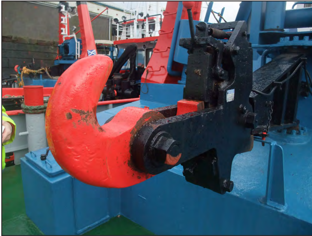
Figure 7: Red Finess - towing hook
