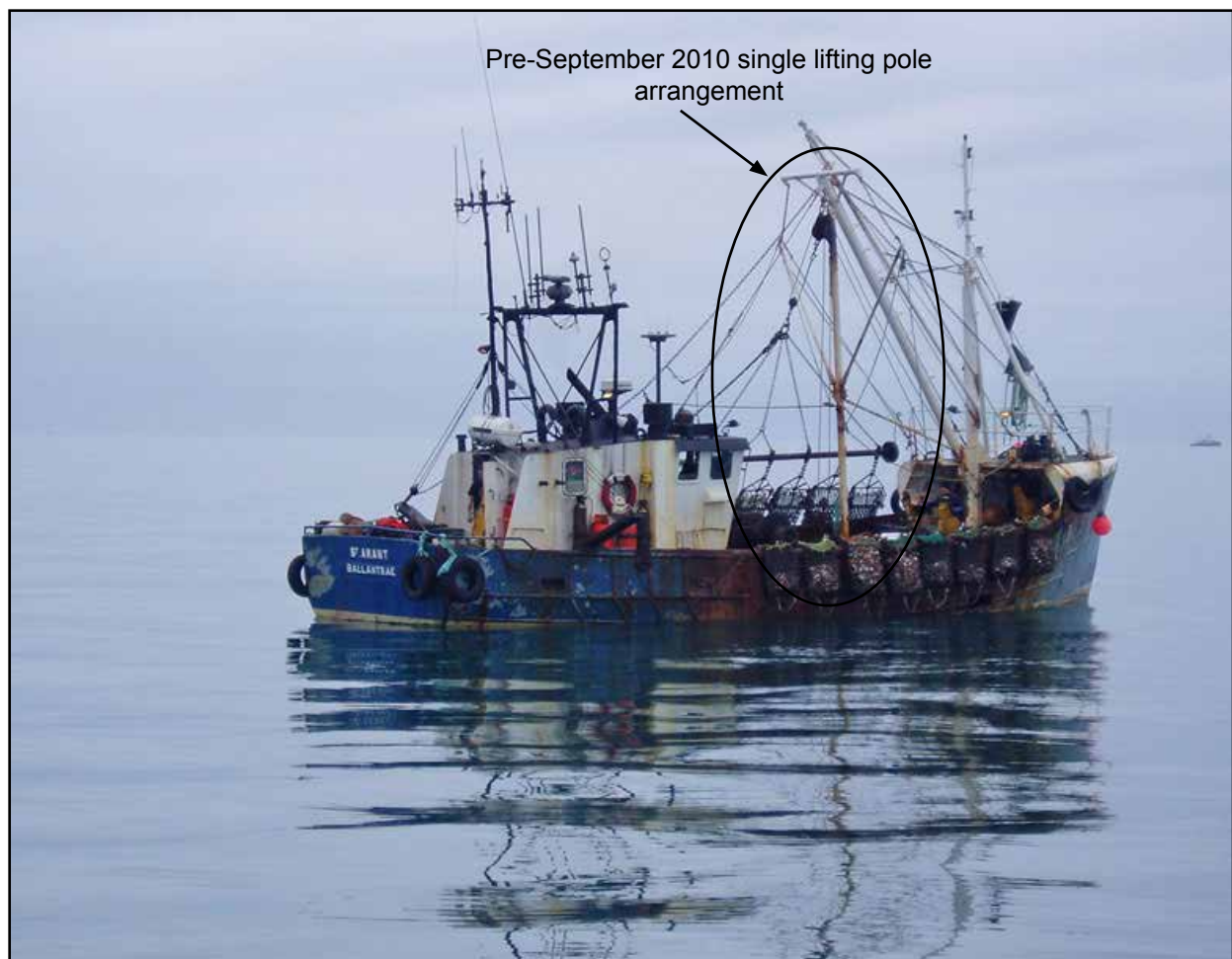
Figure 16a: Lifting arrangement on St Amant before modification in 2010
