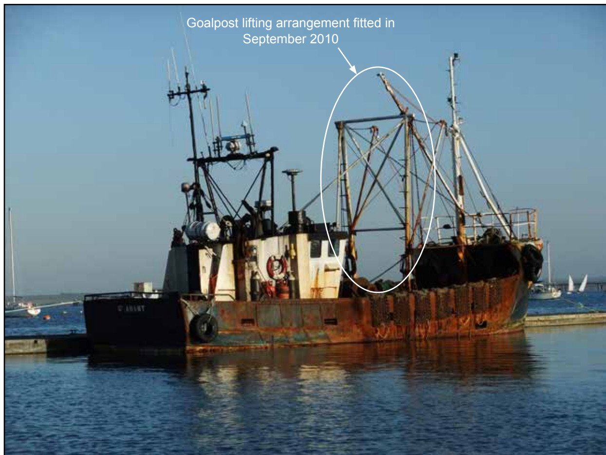
Figure 16b: Lifting arrangement on St Amant after modification in 2010
