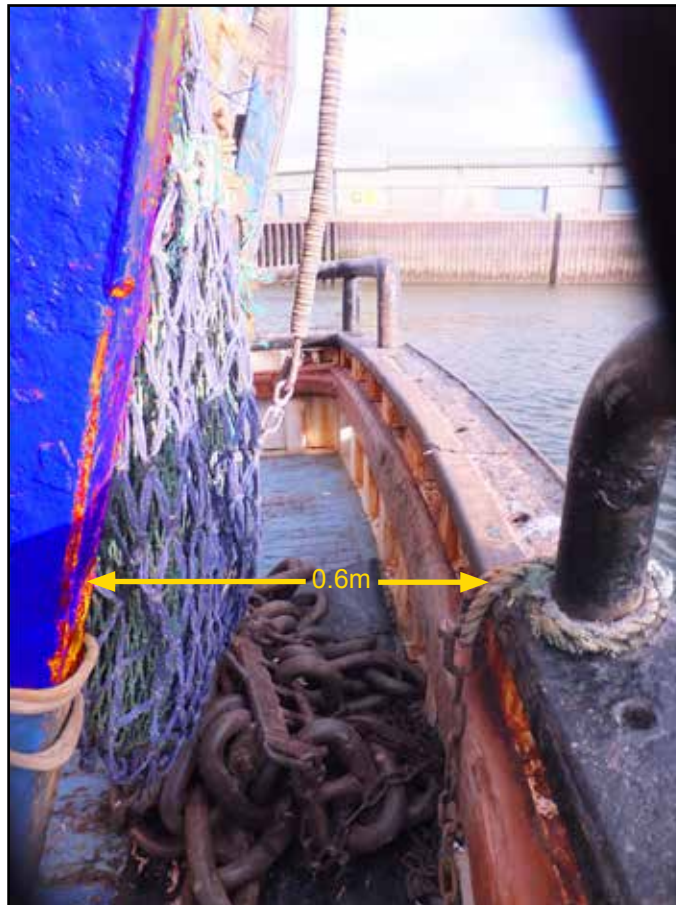
Figure 6: Showing distance between net drum supporting legs and transom = 0.6m
