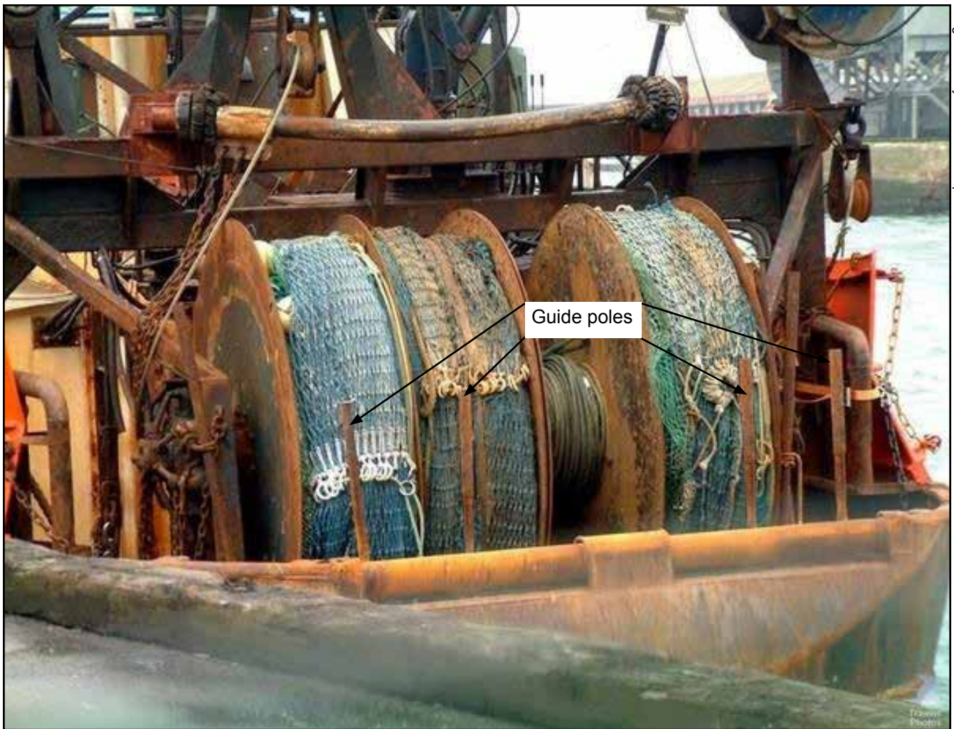
Figure 9: Stern trawler showing example of a deck mounted net drum with guide poles in place
