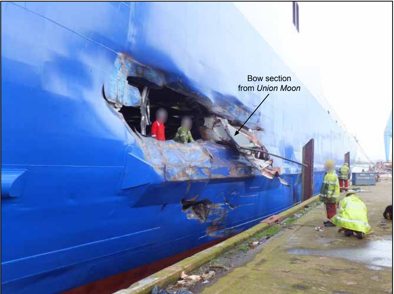
Figure 4: Damage to Stena Feronia
