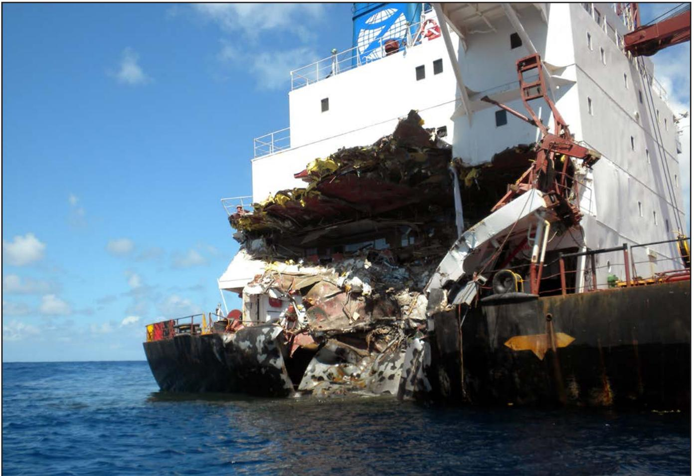
**Figure 13b:** Seagate's starboard side – post-collision (close-up)
