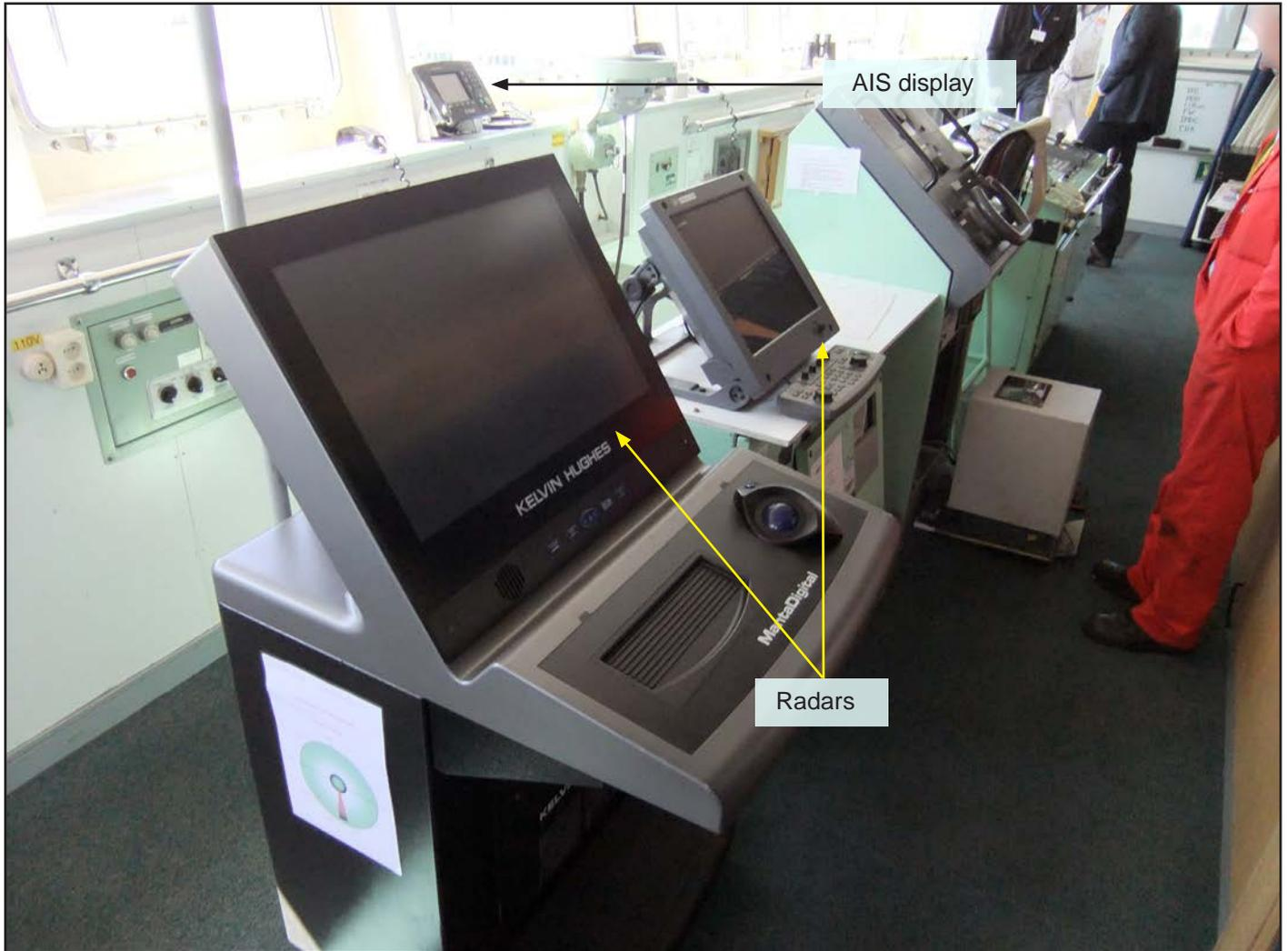
Figure 19: *Timor Stream's* bridge – radars and AIS display
