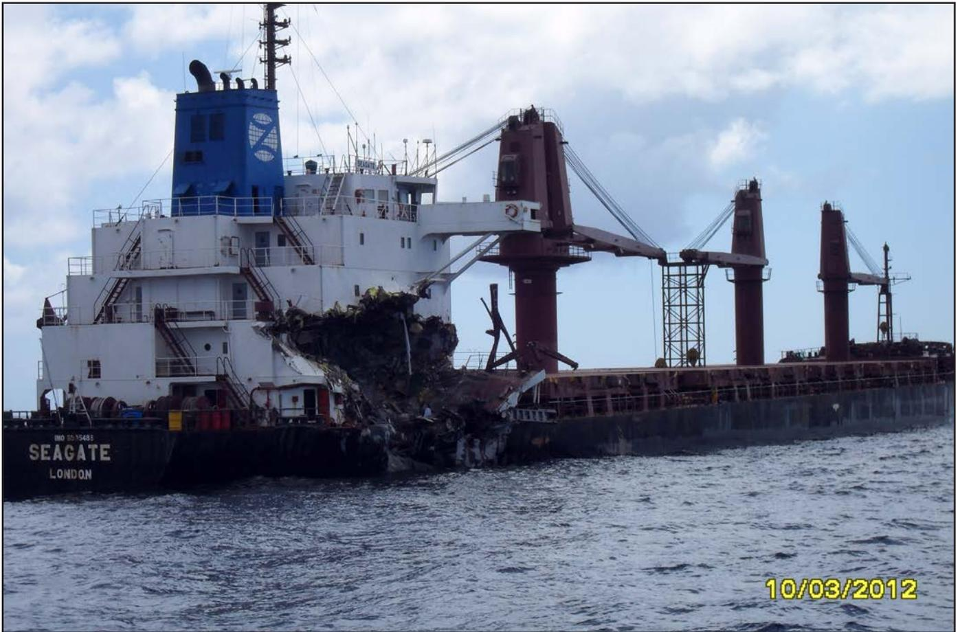
**Figure 13a:** Seagate's starboard side – post-collision
