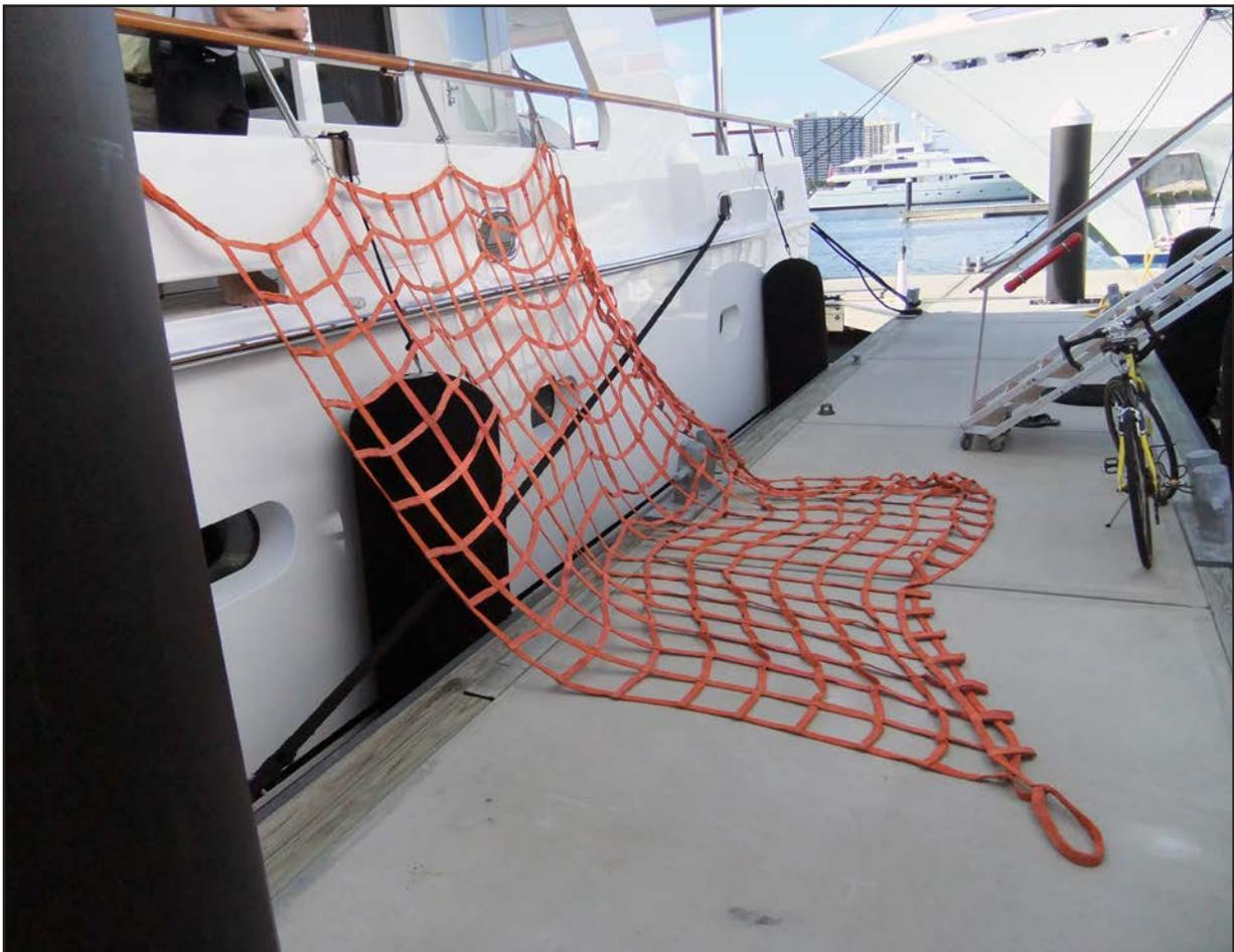
**Figure 11:** *Battered Bull's* manoverboard recovery net
