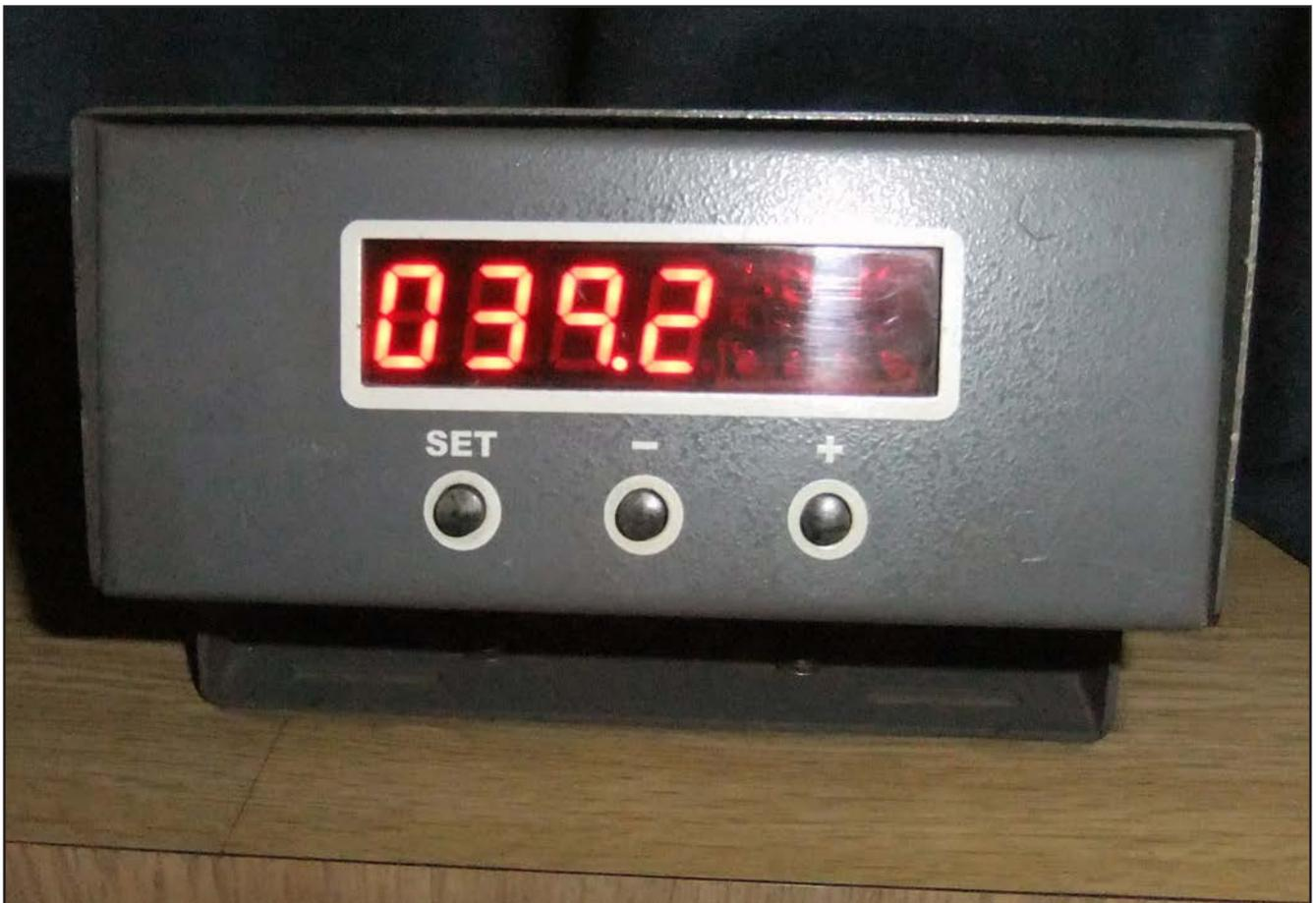
**Figure 22:** *Timor Stream's* gyro interface repeater
