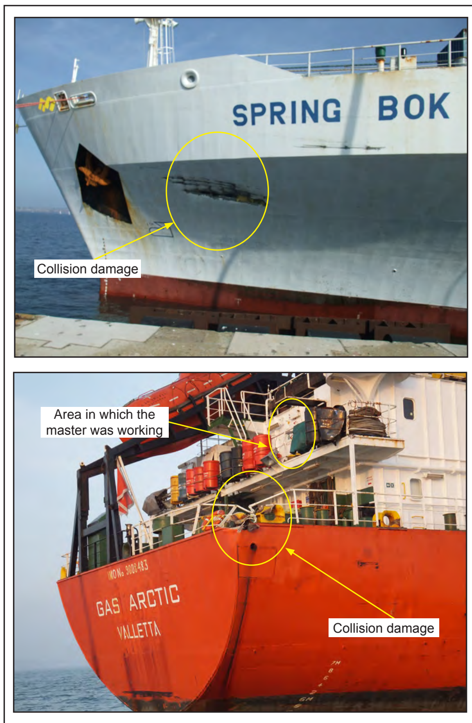
Figure 6: Damage to both vessels
