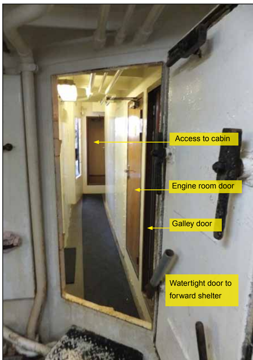
Figure 4: Access to the engine room via a door sited on the port side of the main alleyway ( Ocean Challenge )
