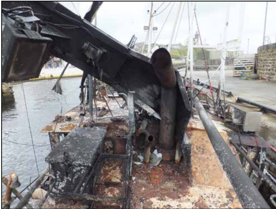
Figures 7: Exhaust exit from deckhouse deckhead
