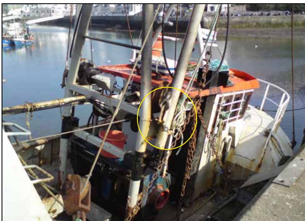
Figure 3: Betty G derrick head block release
