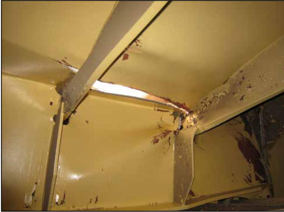
**Figure 11:** UKD Bluefin damage to internal frames
