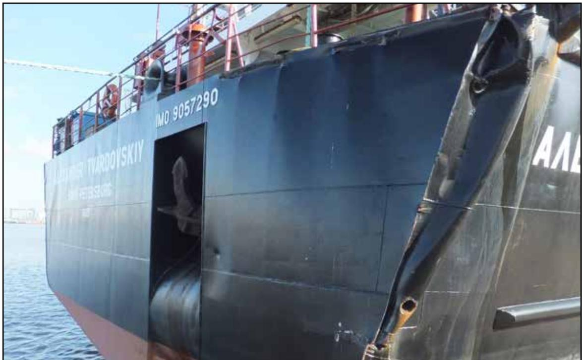
**Figure 8:** *Alexander Tvardovskiy* damage to starboard quarter
