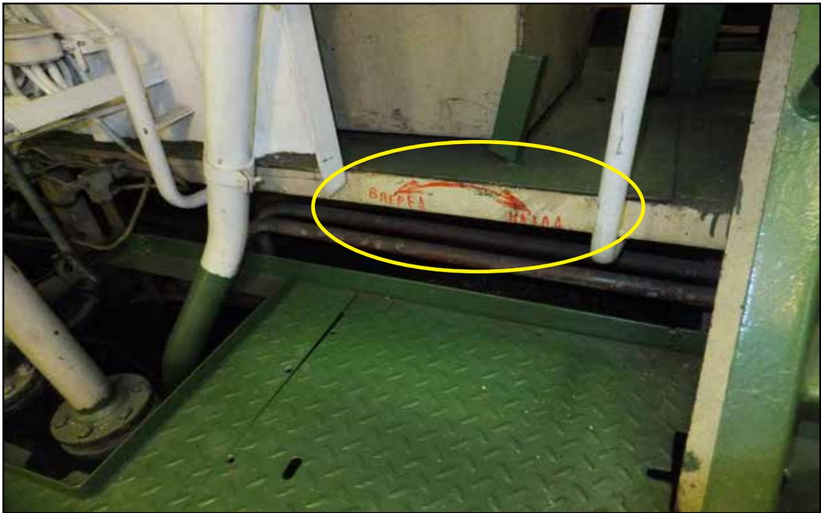
**Figure 26:** Signage showing the direction of shaft rotation in the engine room
