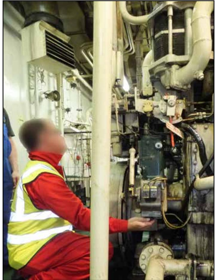
**Figure 25:** Manual control of the main engine speed
