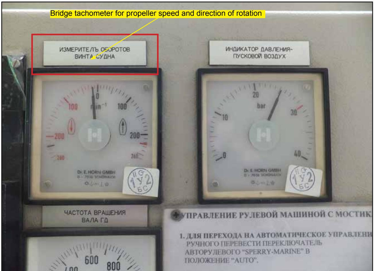
Figure 17: Bridge tachometer for propeller speed and direction of rotation
