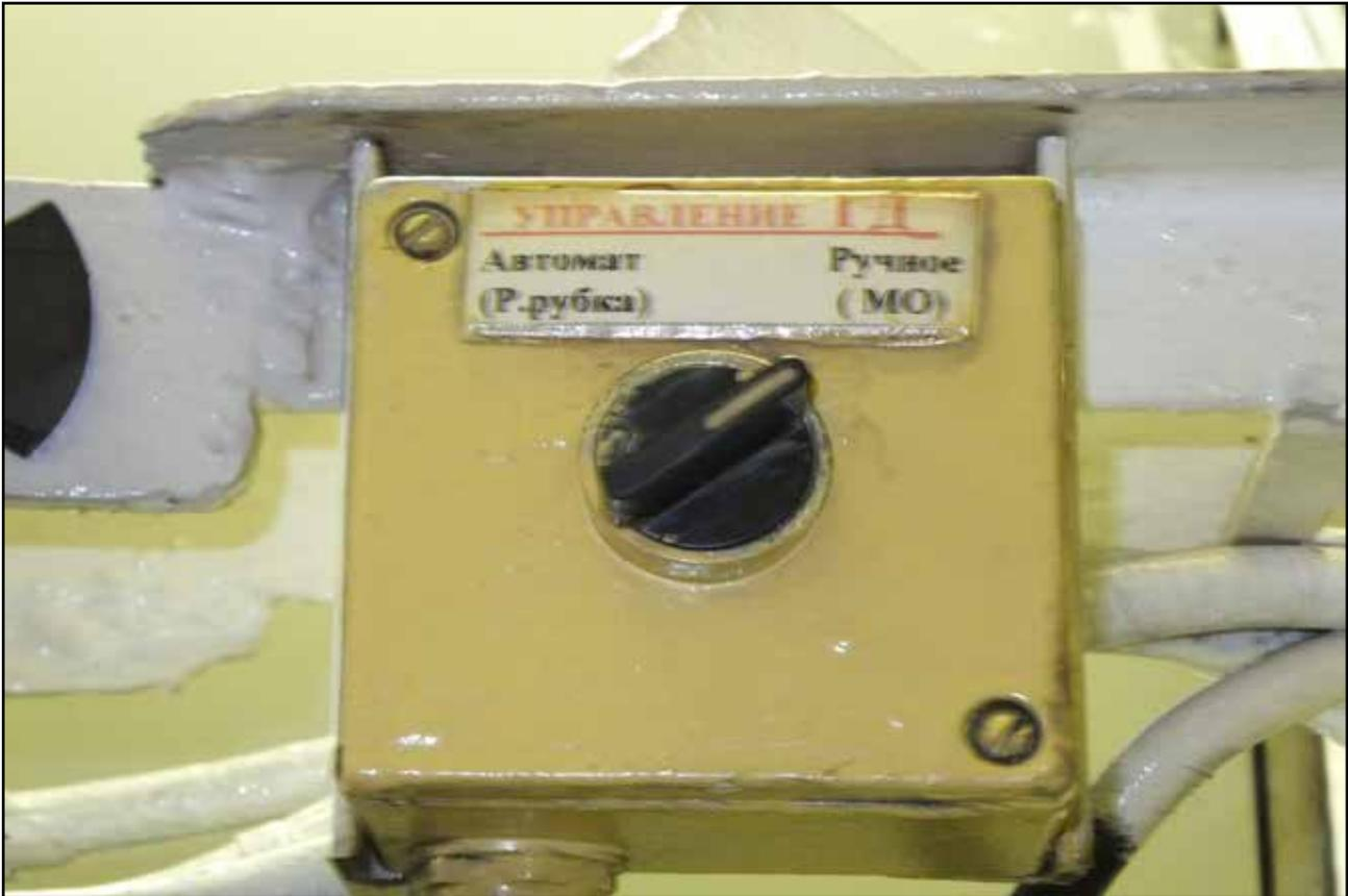
**Figure 18:** Changeover switch: automatic or manual control
