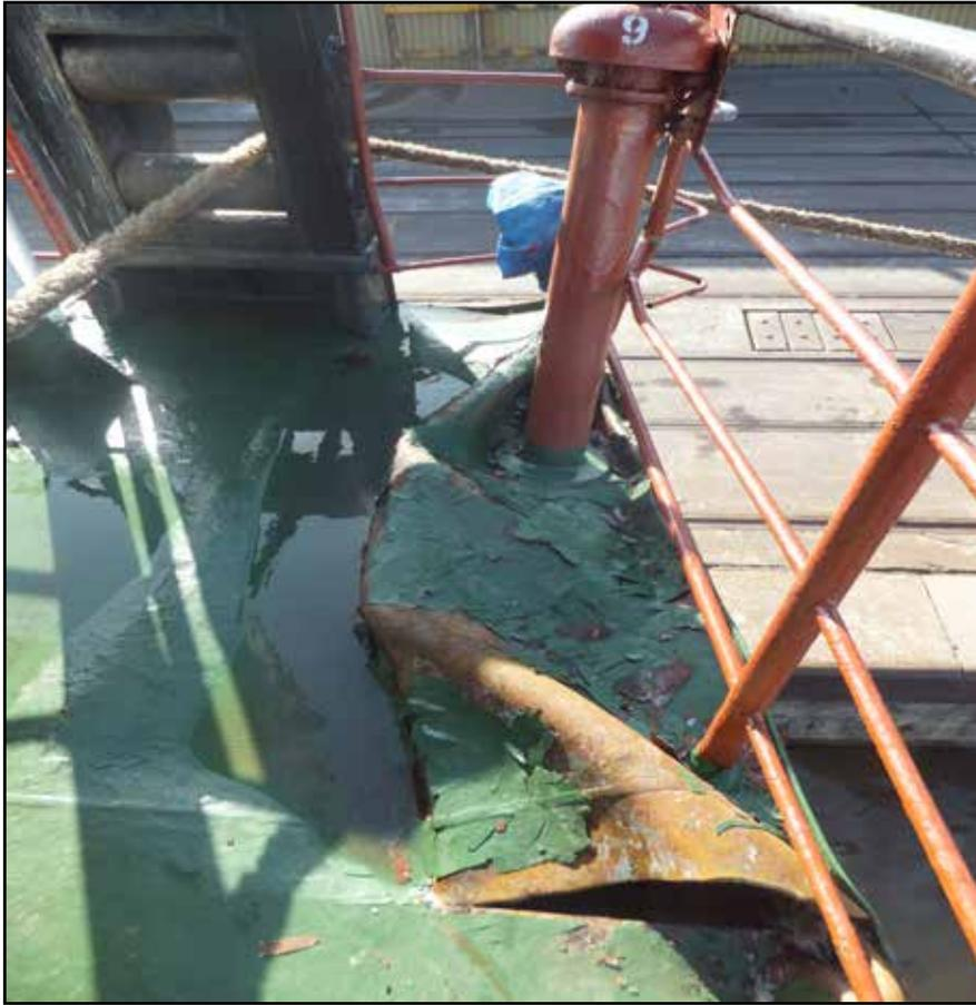
**Figure 9:** *Alexander Tvardovskiy* damage to poop deck
