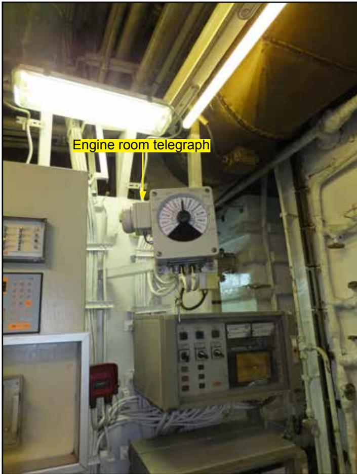
**Figure 24:** Engine room telegraph
