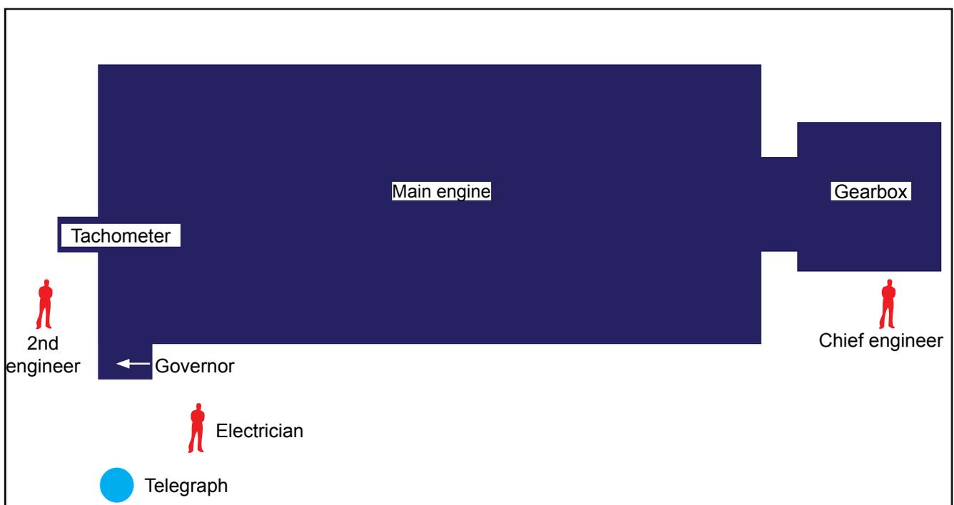
**Figure 23:** Positions of engineers
