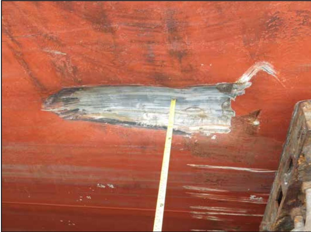
**Figure 13:** *Wilson Hawk* damage to shell plate starboard side
