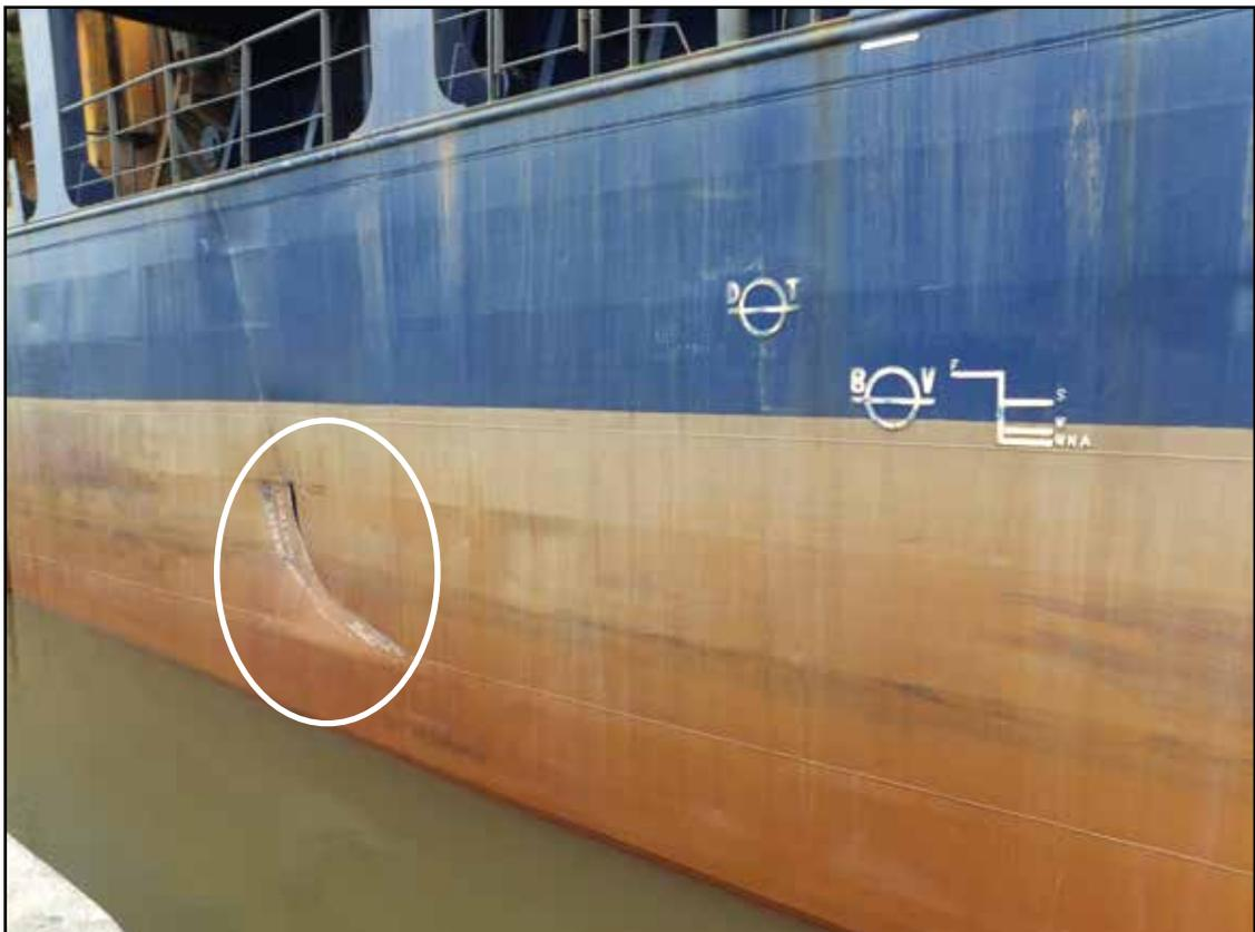
**Figure 10:** *UKD Bluefin* damage to starboard shell plate
