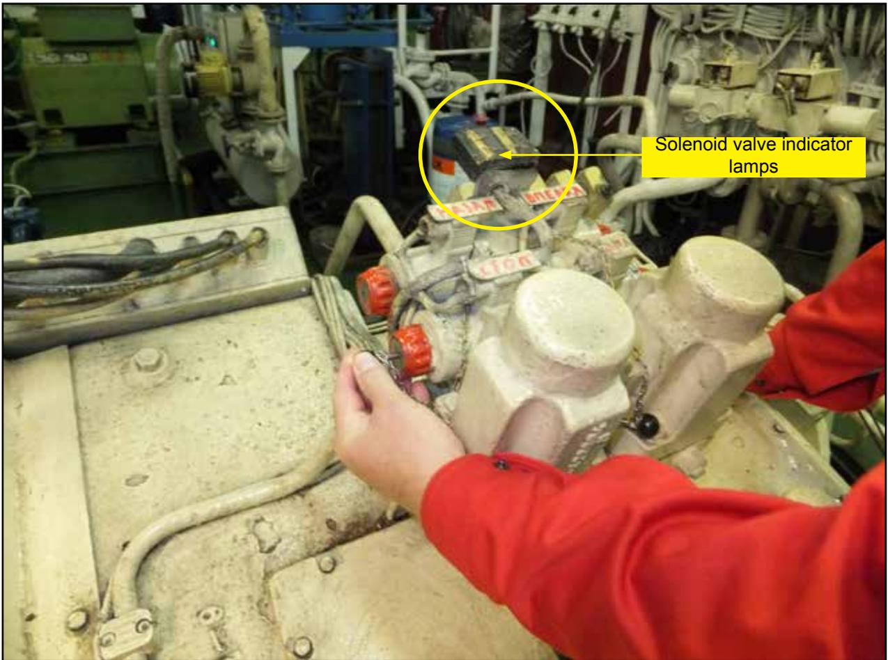
Figure 20: Gearbox solenoid valve block
