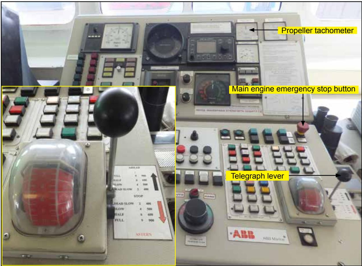
**Figure 4:** Bridge propulsion control panel
