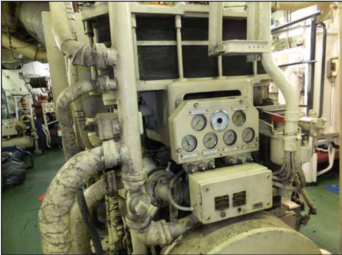
**Figure 15:** Main engine control panel
