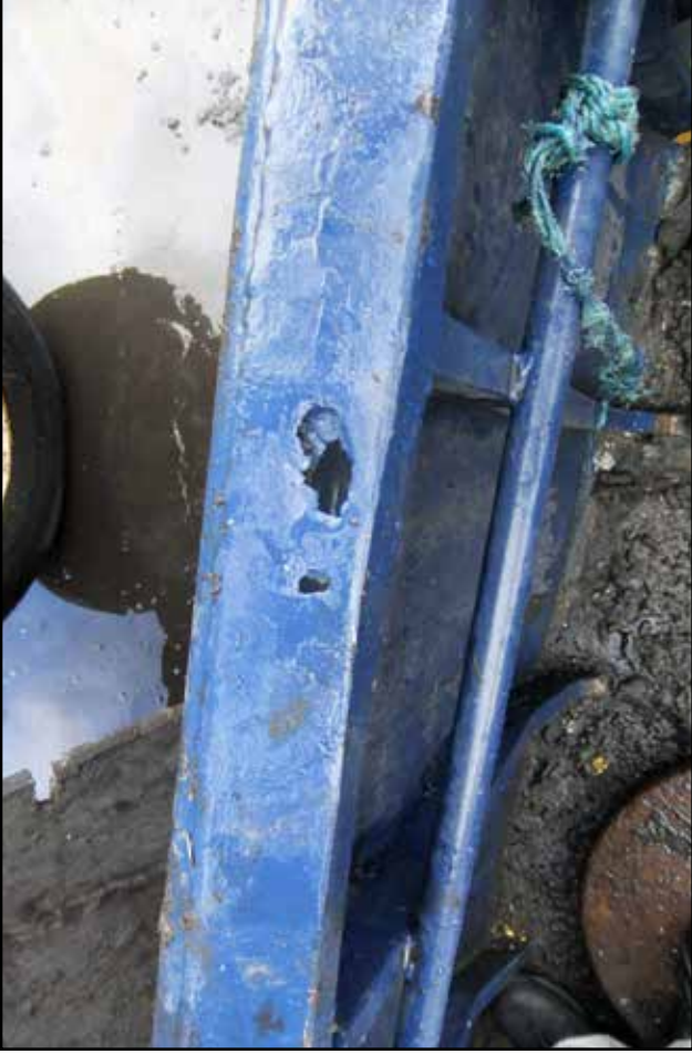
Figure 18b: Gunwhale top corrosion
