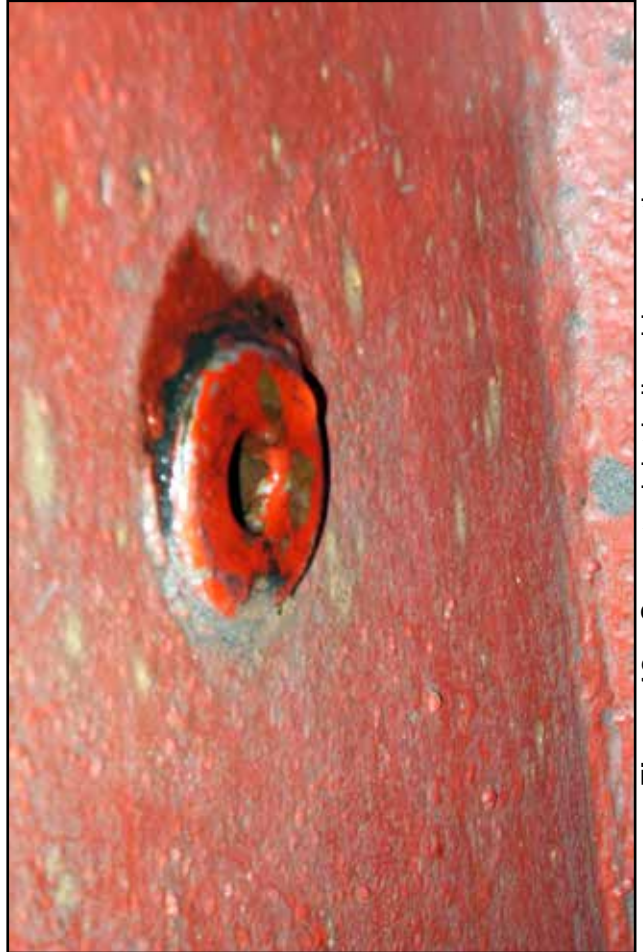
Figure 18a: Hull penetrations above the waterline
