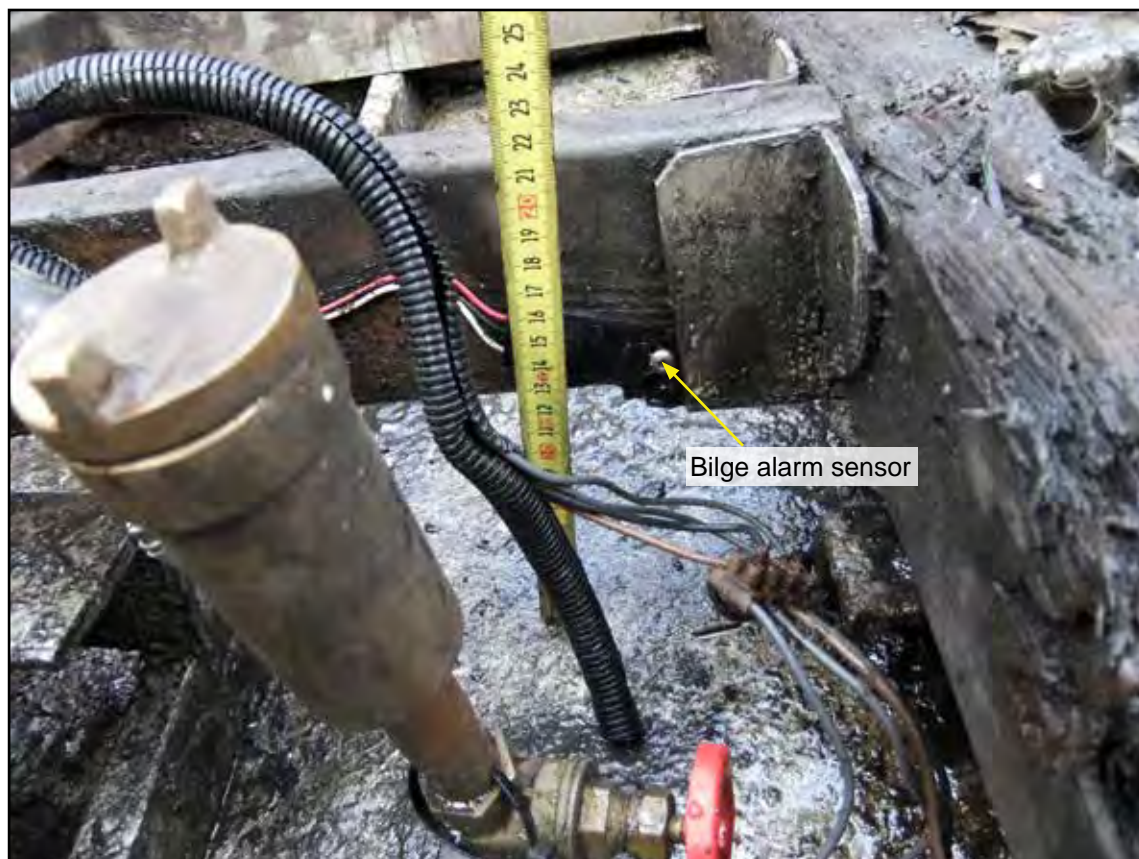
Figure 17: Bilge alarm sensor
