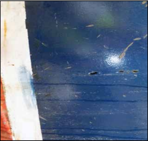
Figure 18a: Hull penetrations above the waterline
