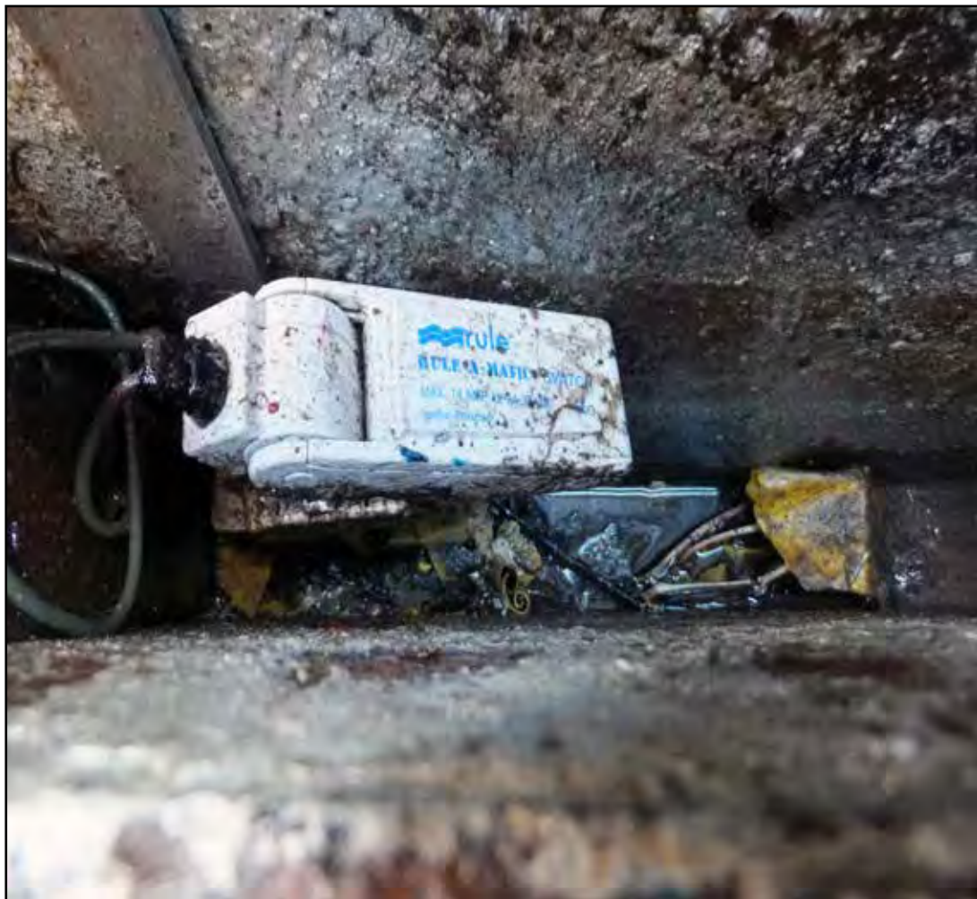
Figure 16: Vixen's bilge and float switch
