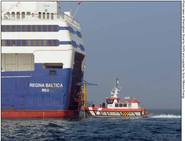
Figure 26: Regina Baltica passenger transfer arrangement
