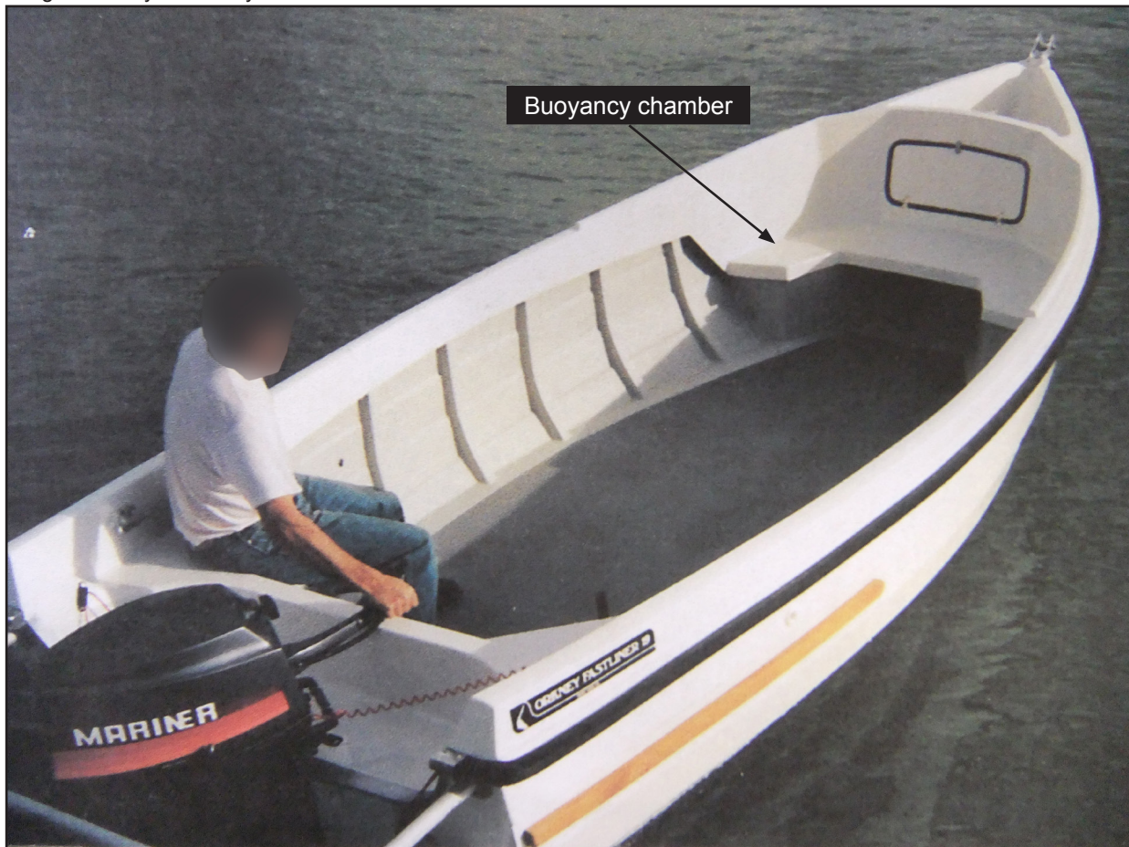
Figure 6: Orkney Boats Ltd, Commercial Model Fastliner 19. Note: no central thwart or side chambers
