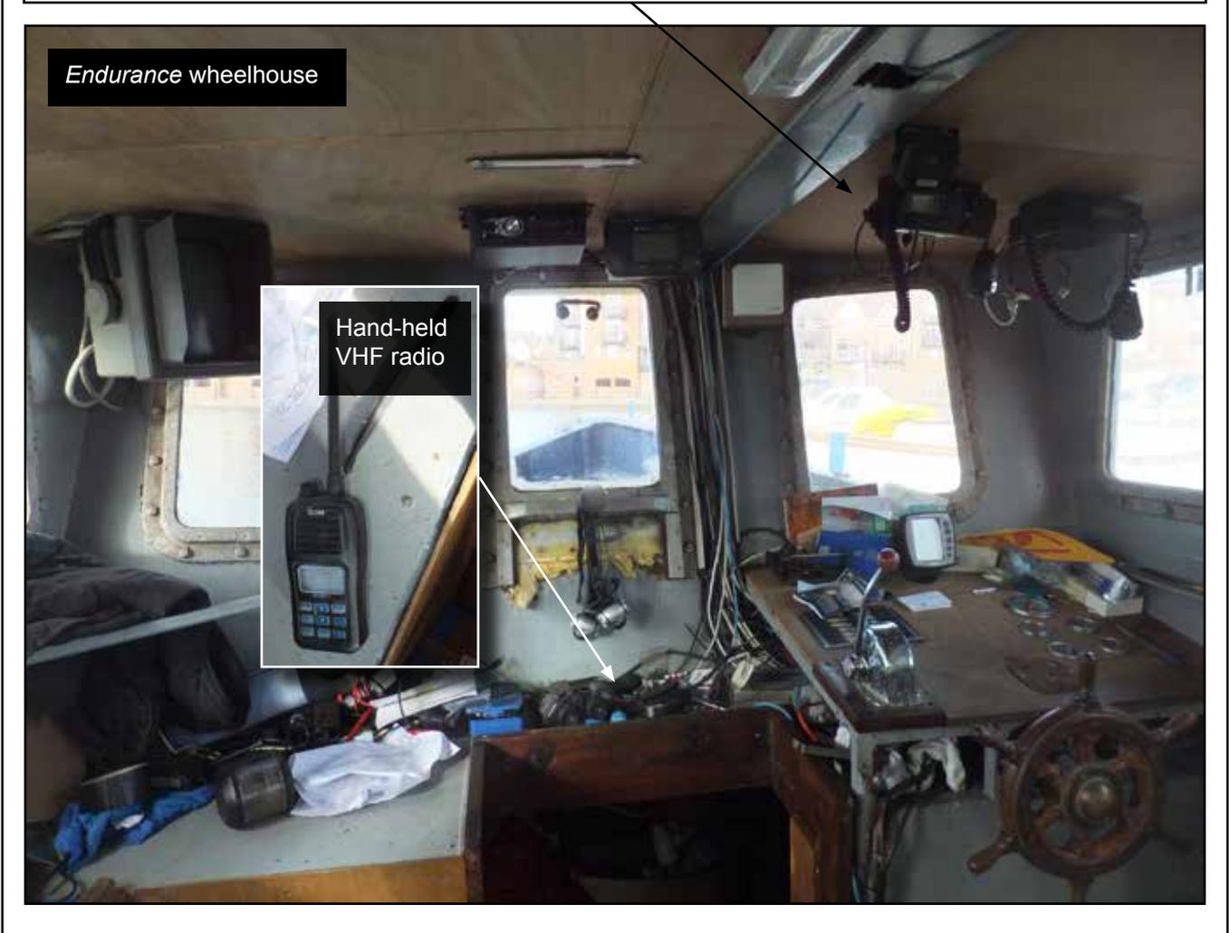
**Figure 18:** Combined VHF and DSC radio fitted on board *Endurance*
