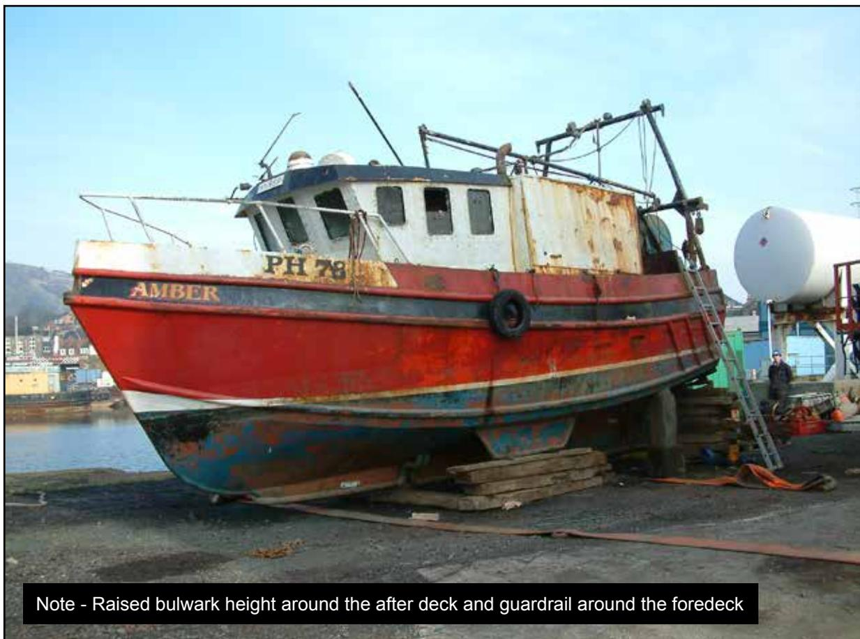
Note - Raised bulwark height around the after deck and guardrail around the foredeck
