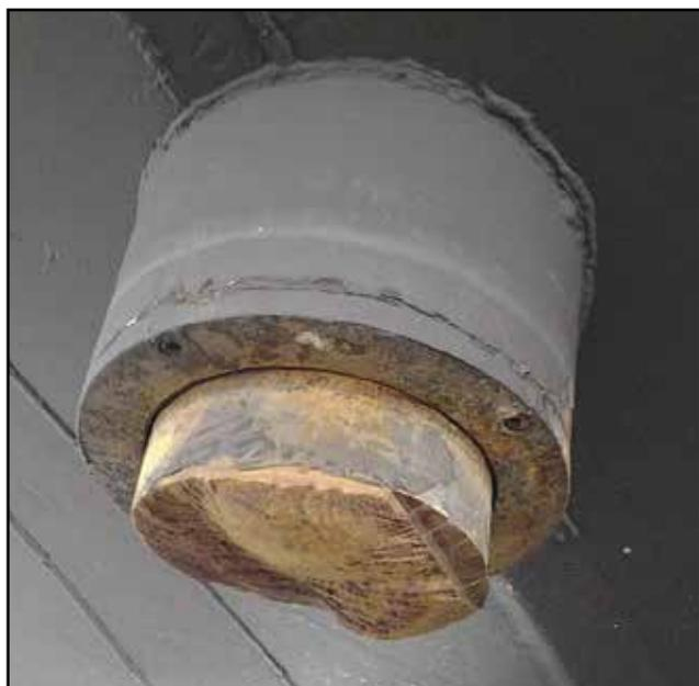
**Figure 4:** Broken rudder stock
