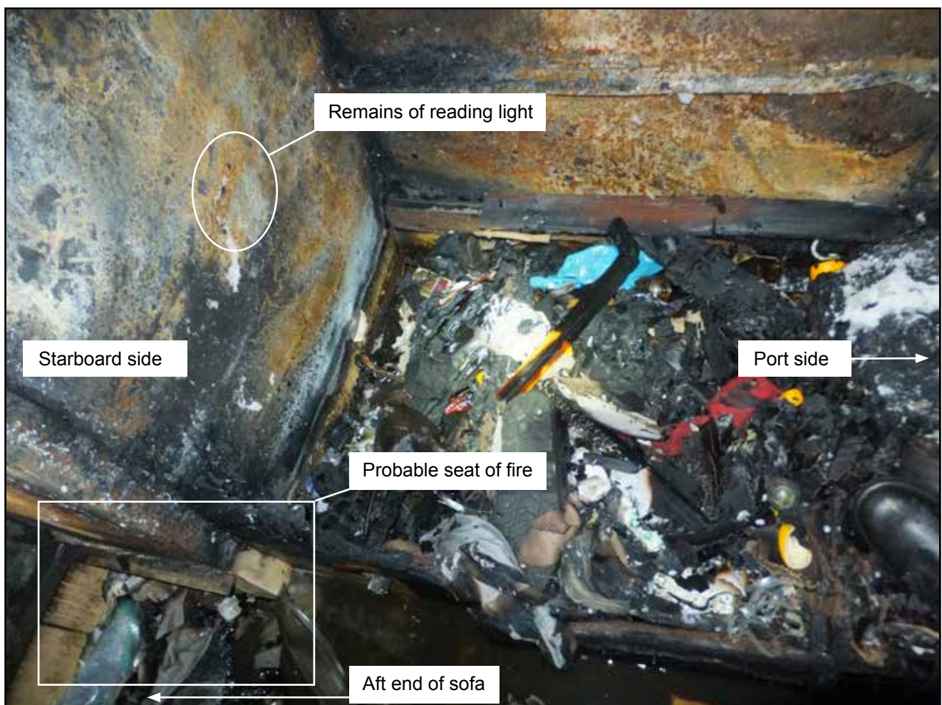
Figure 6: AB2's cabin fire-damaged bunk
