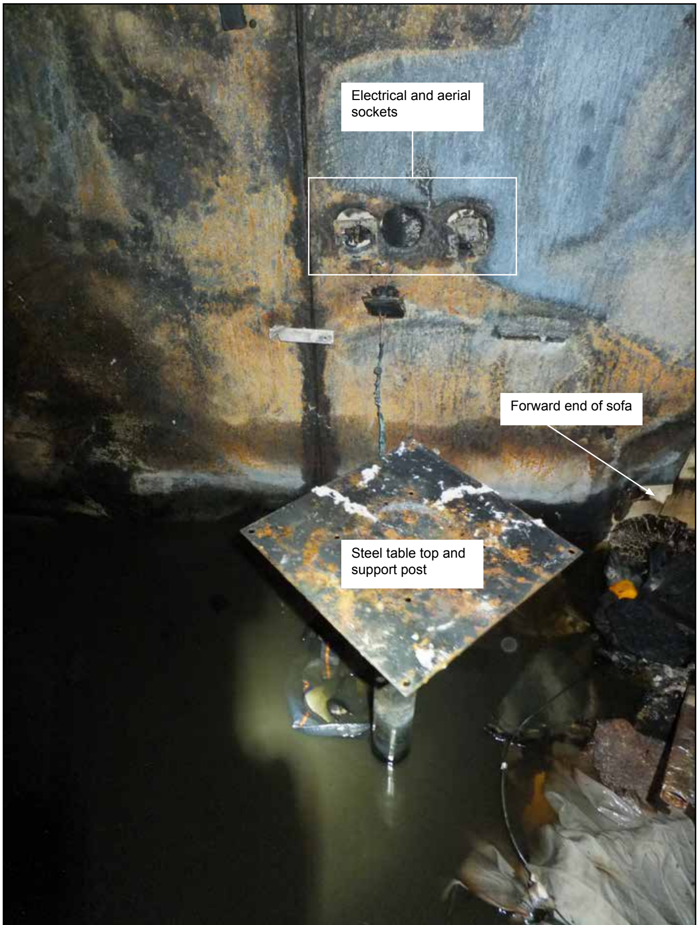
Figure 7: AB2's cabin fire-damaged table
