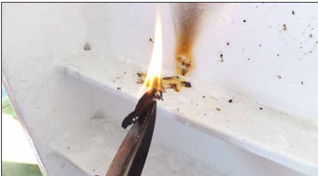
Figure 11: Cabin mattress and sofa ignitability test
