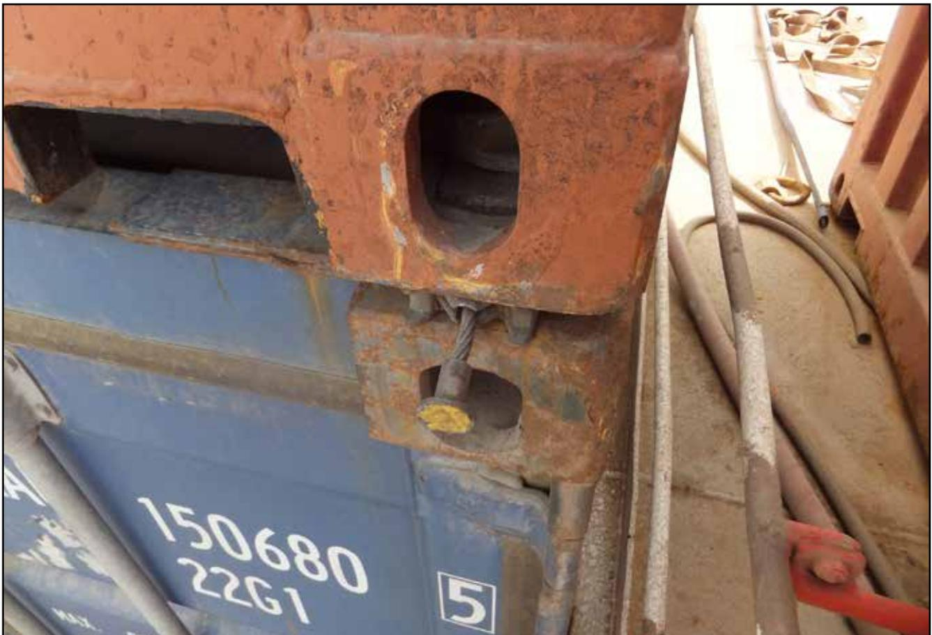
**Figure 7:** Semi-automatic twistlock securing two containers together
