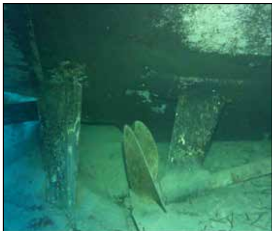
Figure 3: Isamar 's starboard propeller and bracket (intact)
