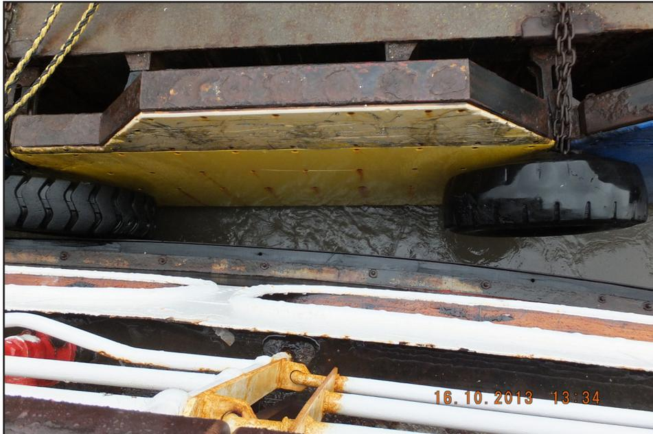
**Figure 5:** Gap between *Snowdrop* and Seacombe terminal fendering
