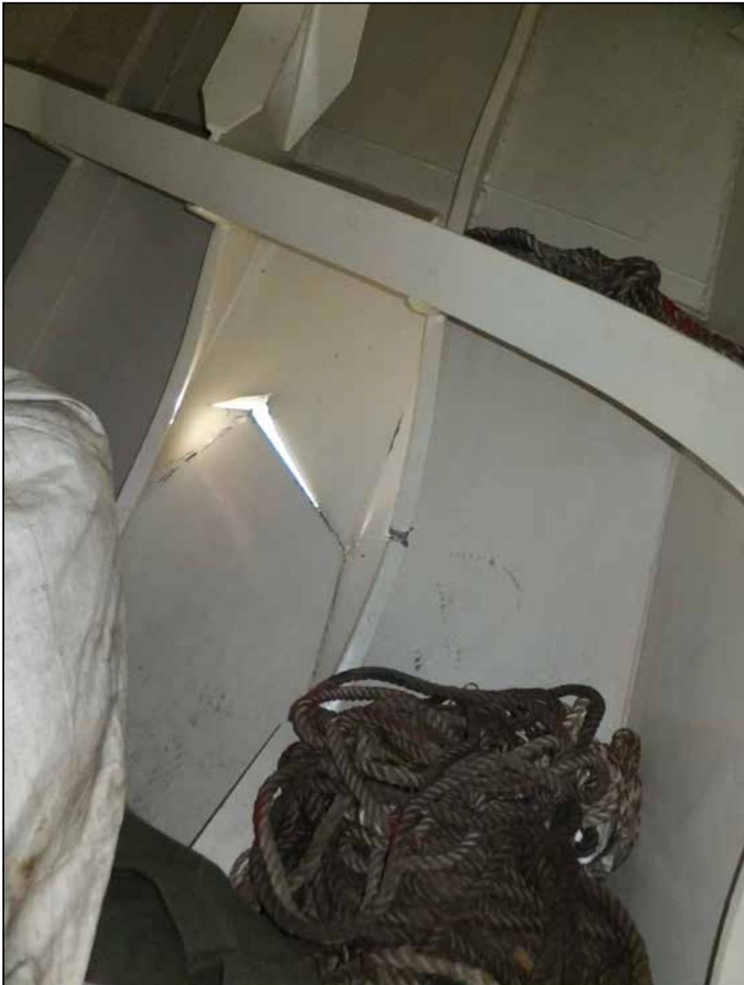
**Figure 6:** *Rickmers Dubai* - collision damage (internal)
