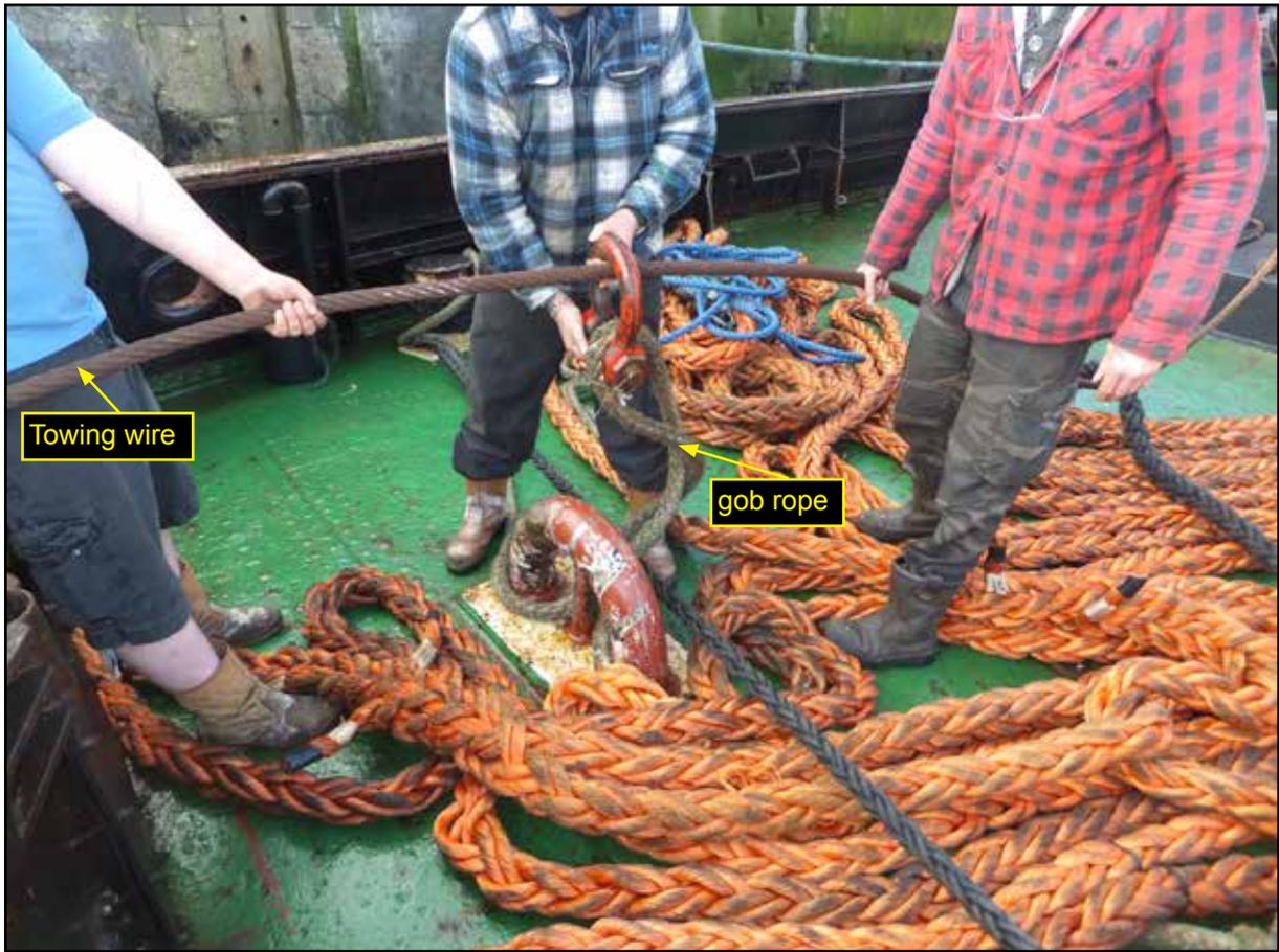
**Figure 13:** Kingston - gob rope arrangement
