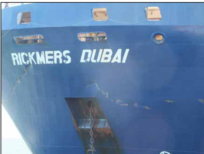
**Figure 5:** *Rickmers Dubai* - collision damage (external)
