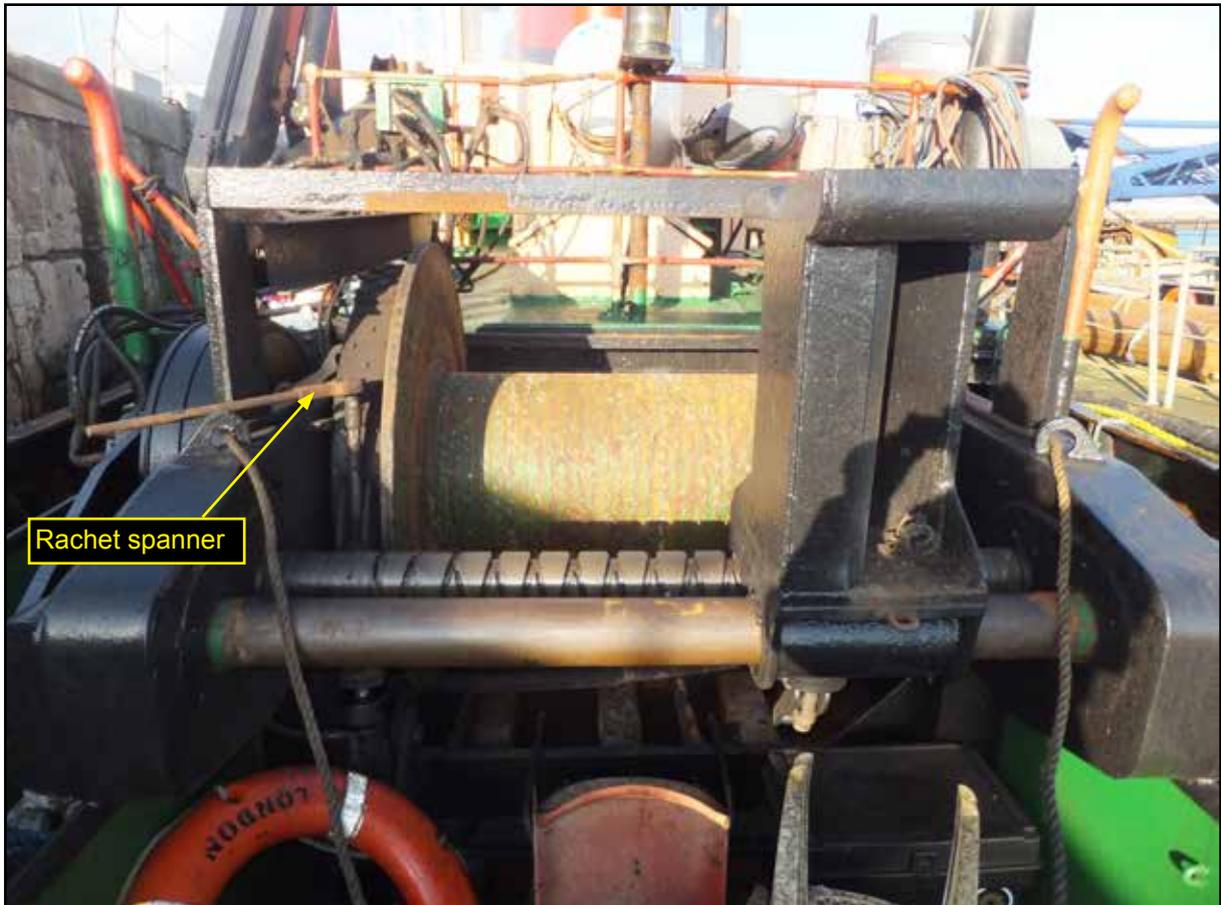
**Figure 14:** Kingston - towing winch
