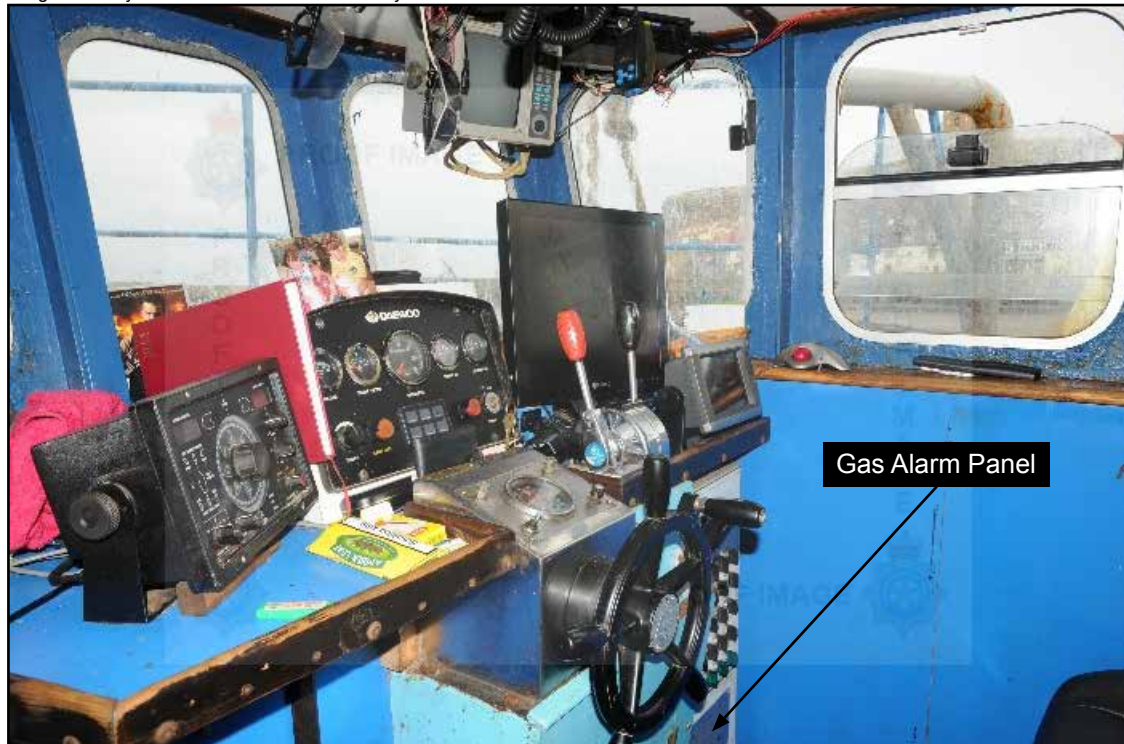
Figure 6: Wheelhouse control console
