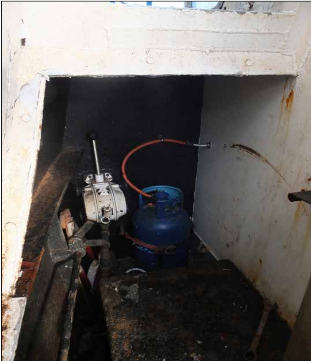
Figure 13: Butane gas cylinder stowage
