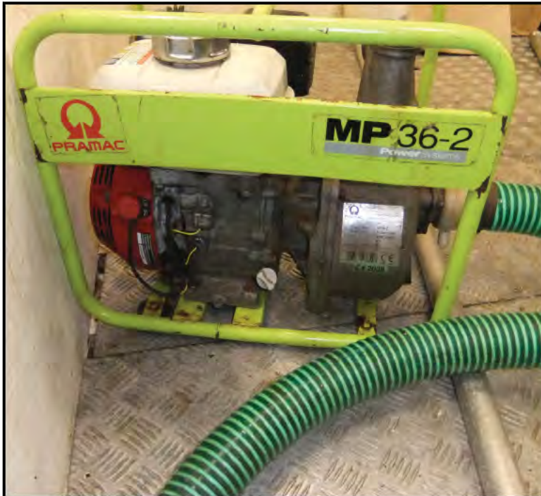
Figure 1: The petrol engine-driven salvage pump
