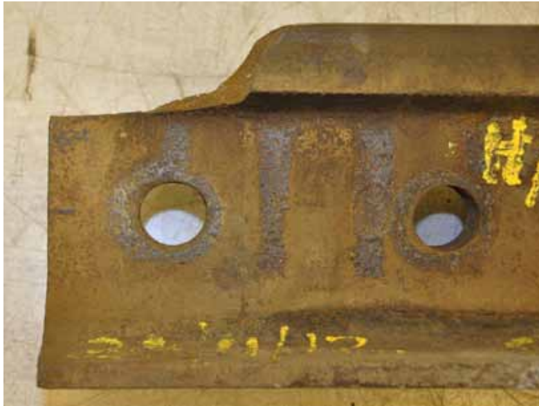
Rail with broken portion missing and fishplate removed
