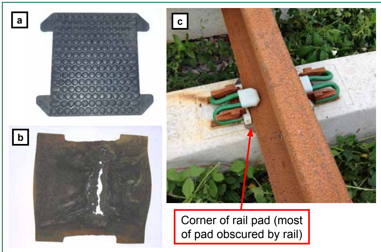
Figure 29: Rail pads in (a) new condition, (b) worn condition and (c) fitted beneath rail
