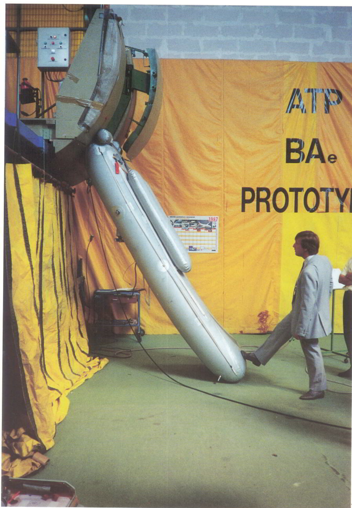
FIGURE 6 - THE SLIDE FROM G-PEEL FITTED TO THE MOCKUP AND DEPLOYED AT MAXIMUM SILL HEIGHT, I.E. NOSE GEAR COLLAPSED.
