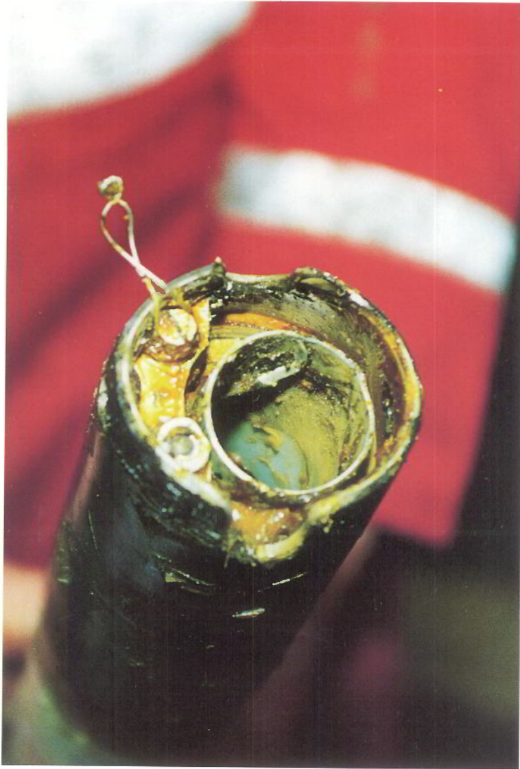
FIGURE 4 - LEFT. THE BAULK DEVICE PUSHED INTO THE PINTLE PIN, AS FOUND
