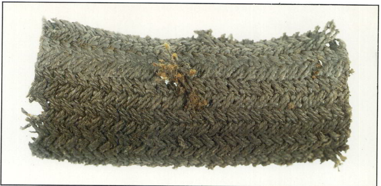
Hose outer layer covering area of rupture
