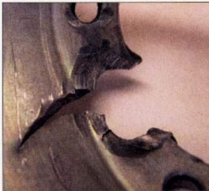
Figure 3: Failed wheel half showing typical overload failure originating at edge of wheel mounting hole
