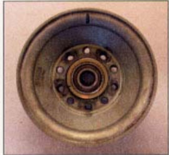
Figure 2: Undamaged wheel half overlaid on top of hub, showing alignment of holes in wheel with holes in hub. (Alignment mark on wheel rim was made subsequently by the AAIB)
