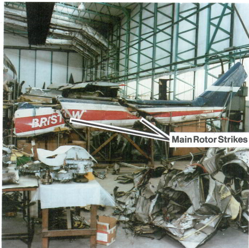
2. G-BJJR Tail boom showing main rotor strikes.
