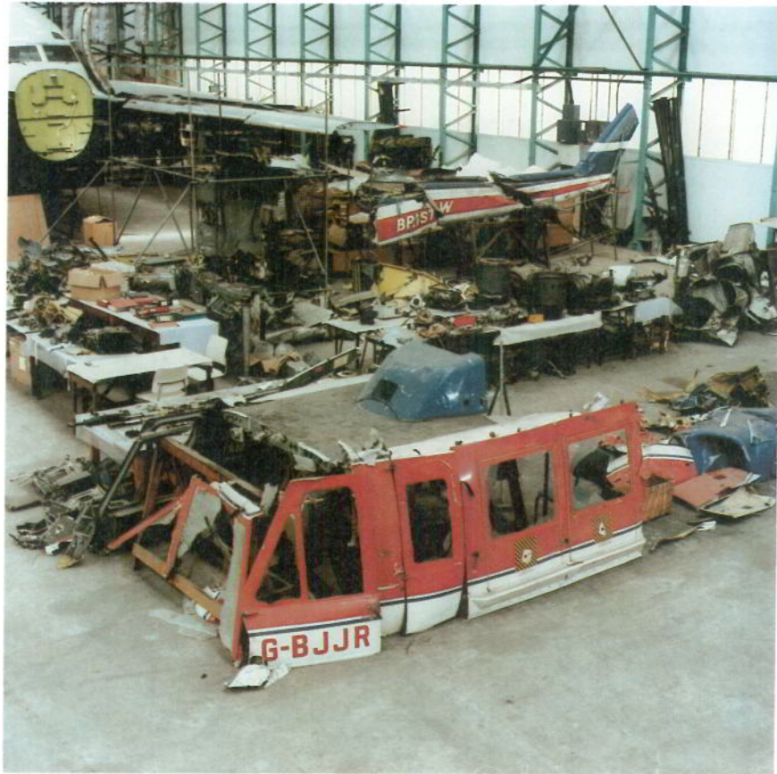
1. G-BJJR Wreckage showing extent of structural disruption.
