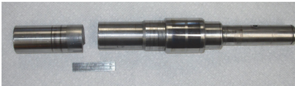
Figure 4 The two pieces of the shaft after removal from the aircraft
