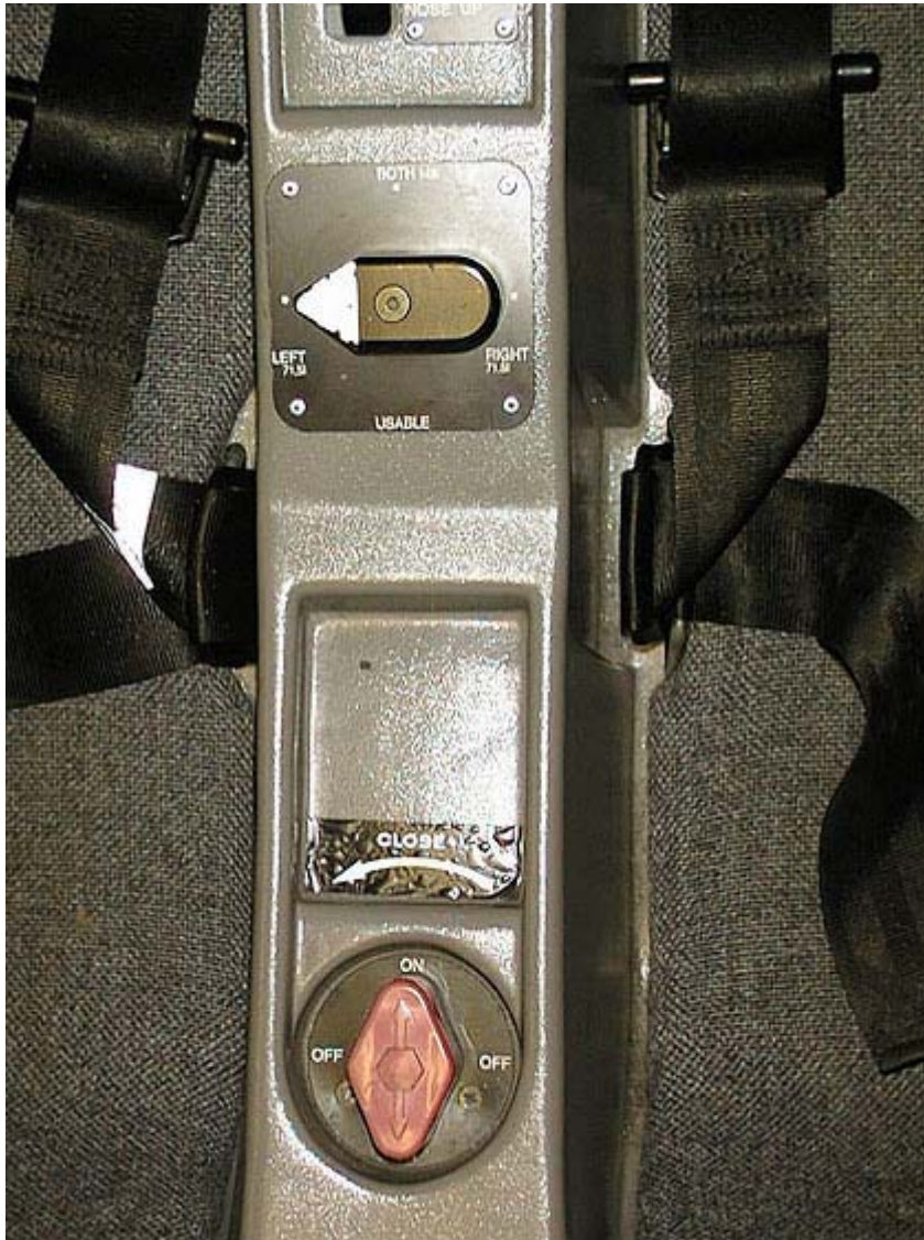
Figure 3 - Fuel tank selector and ON/OFF cock locations in later models
