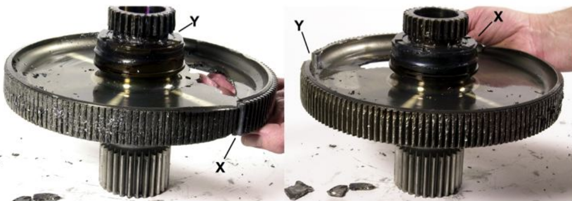
Figure 7 Pattern of post-fracture tooth damage
