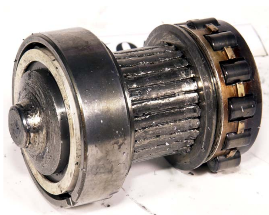
Figure 5 Input (high speed) pinion, showing sheared drive neck
