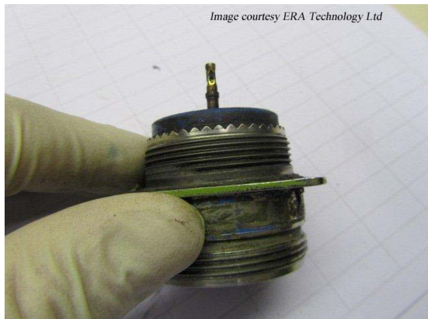
Figure 1 D1114J connector, showing the detached crimp terminal at pin 12
