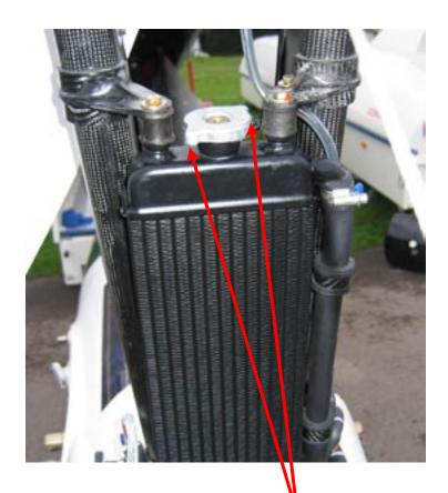
Note: Lugs of cap only just pass upper radiator mounts. Cap shown in fully closed position.
