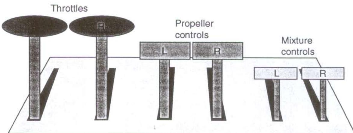
Figure 2: Conventional engine control layout
