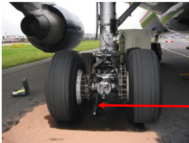
Disconnected brake reaction rod
