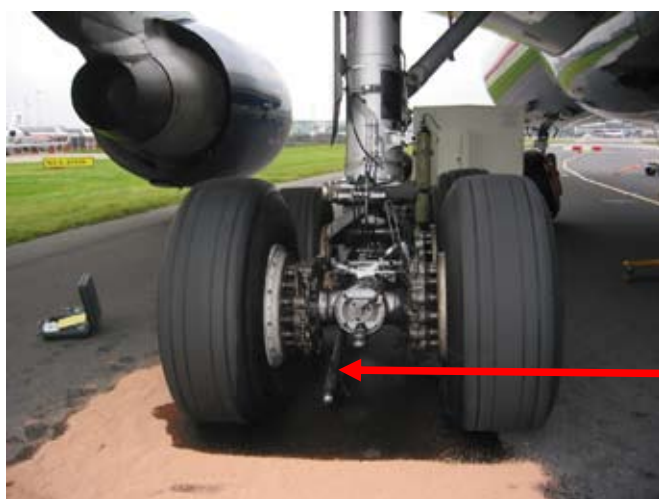
Disconnected brake reaction rod
