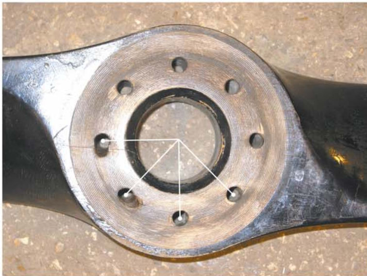
Figure 2:- Aft face of left propeller (note elongated holes)
