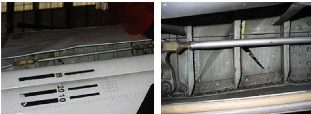
**Figure 5** Structural damage to upper wing skin and rear spar
