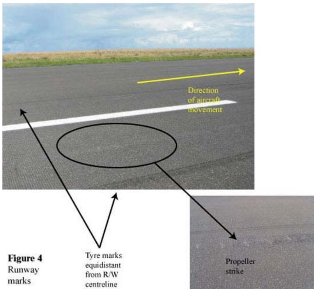
The groundspeed at the time the propeller strikes were made was estimated to be 96 kt using the formula given in the ICAO Manual of Accident Investigation and assuming 94% propeller RPM at the second touchdown.
