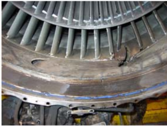
Second stage assembly removed - casing penetrations at 5-7 o'clock positions
