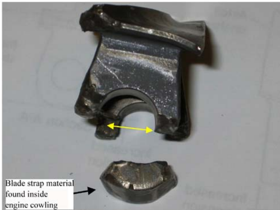
Figure 2 LP compressor second stage blade failure
