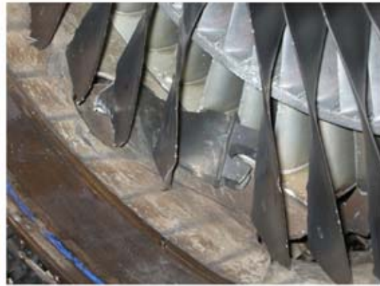
Second stage fan assembly - 'as found' position of detached blade
