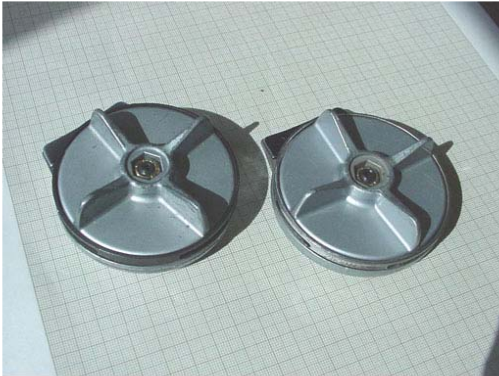
Figure 1 - Failed buckle and example buckle
